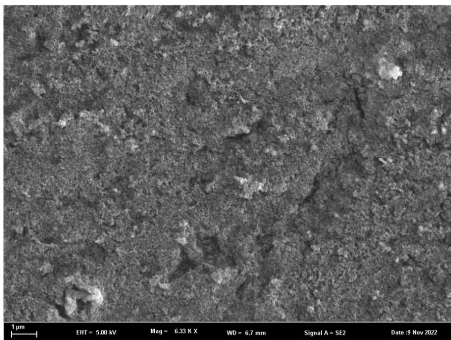
**Figure S7.** The SEM image of the PmPD membrane surface.
