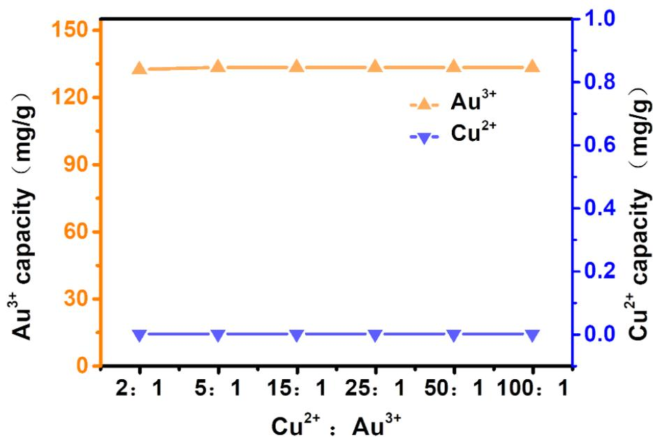
Figure S4. Recovery of Au(III) at different mass ratios of Cu and Au.
