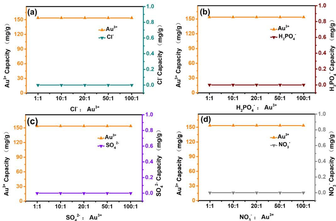
Figure S5. Recovery of Au(III) and coexisting anions by PmPD particles from water containing all ions in different concentrations: removal capacity of Au(III) as compared to Cl<sup>-</sup> (a), H<sub>2</sub>PO<sub>4</sub><sup>-</sup> (b), NO<sub>3</sub><sup>-</sup> (c), SO<sub>4</sub><sup>2-</sup> (d). The concentration of Au(III) was added in 50 mg/L.
