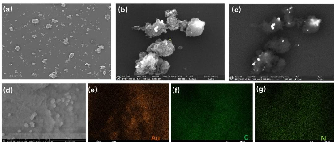
**Figure S6.** SEM and EDS images of PmPD before and after Au(III) adsorption; (a) SEM general images of PmPD before adsorption Au(III) ; (b-c) SEM images of PmPD after adsorption Au(III) ; (d-g) EDS elements distribution of Au, C, N after Au(III) adsorption.
