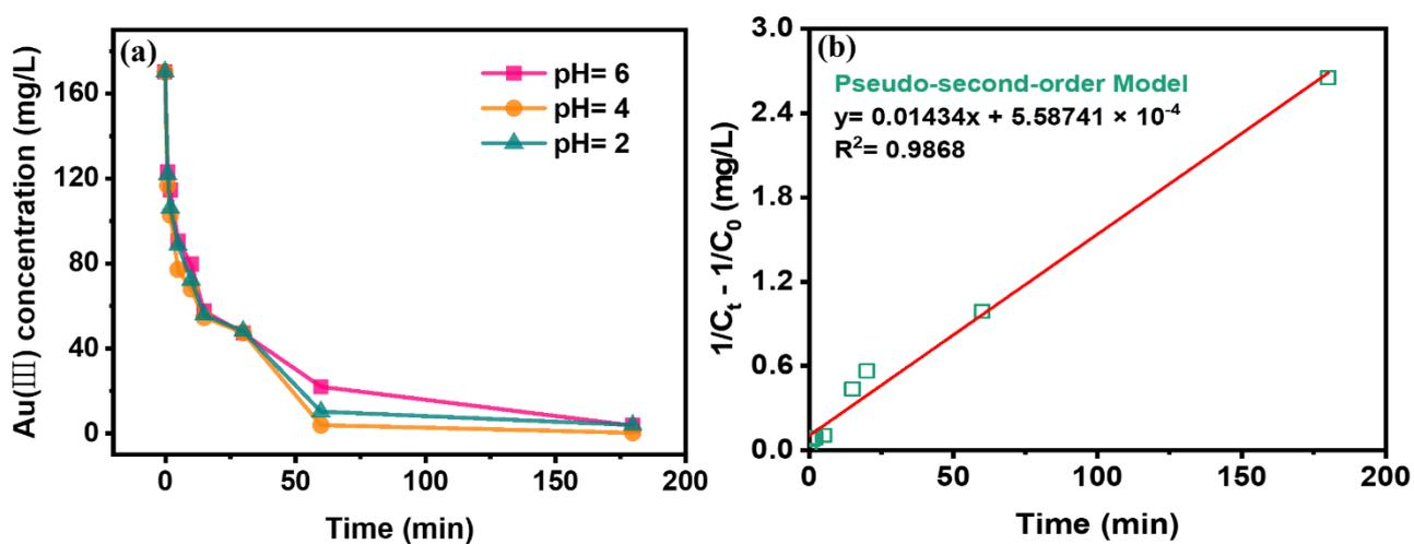
**Figure S2.** Effects of pH on the Au(III) adsorption by PmPD particles, with initial Au(III) concentration of 160 mg/L. (a) adsorption isotherms; and (b) linear fitting by Second-order kinetics model at pH 2.
