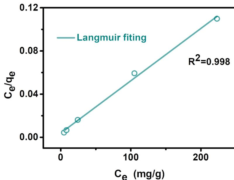
**Figure S3.** Langmuir model fitting for the Au (III) adsorption isotherm.
