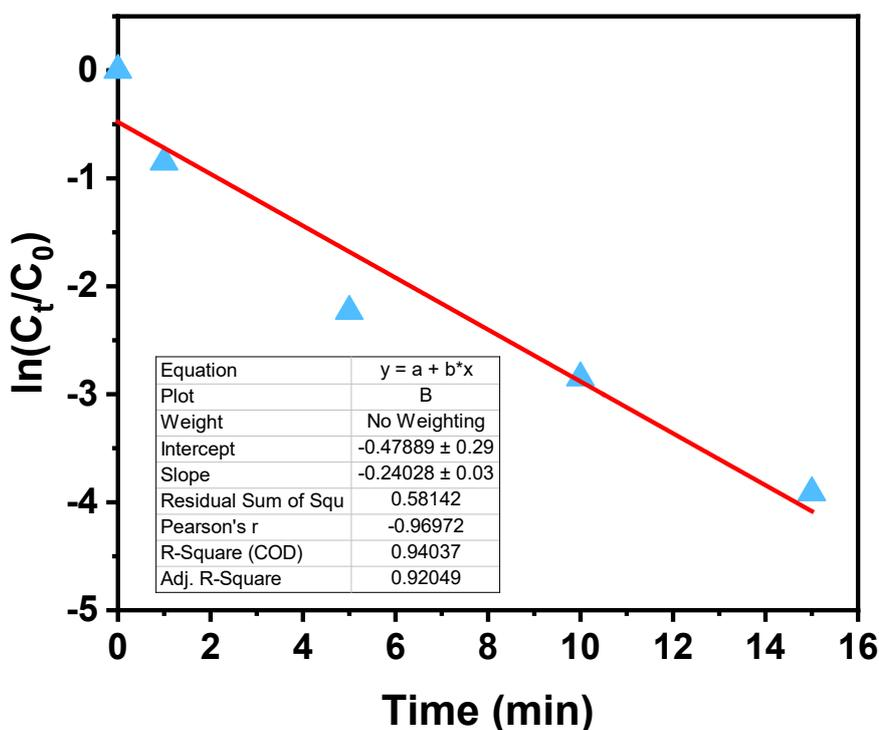
**Figure S8.** Plot of 4-NP concentration evolution  $\ln(C_t/C_0)$  versus reaction time as obtained from the dispersion of Au@PmPD.
