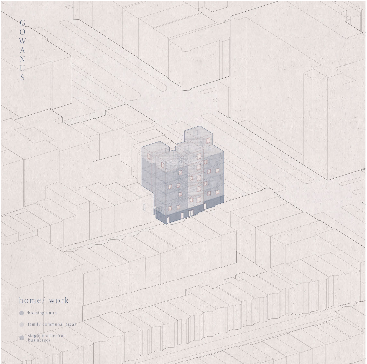
Figure 60. Program massing for a new construction, including businesses on ground floor, and housing on either side connected by a central vertical core.
