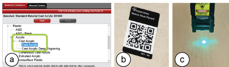
Figure 3-1: Existing material identification approaches: (a) Manually selecting from a database (e.g., ULS [135]) or (b) scanning QR code stickers on sheets ( Glowforge ). (c) SensiCut uses speckle sensing to identify the material based on its surface structure without the need for additional tags.
