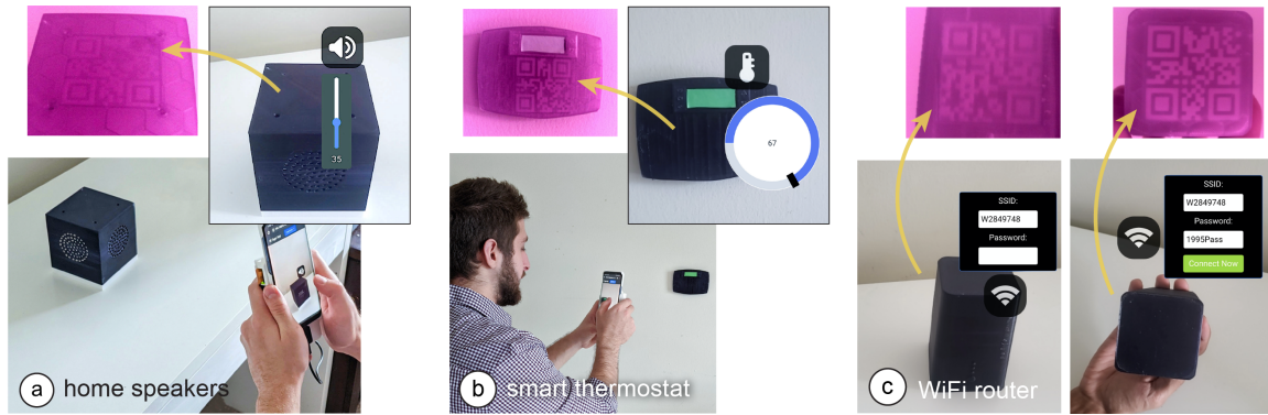
Figure 6-6: Controlling appliances using a mobile AR application. The user points at (a) the home speakers to adjust its volume, and the (b) thermostat to adjust the temperature. The infrared camera in the phone’s case identifies the appliances by reading the embedded QR codes. (c) Pairing a phone with a WiFi router, whose SSID is visible from all sides but the password is visible only from its bottom.
