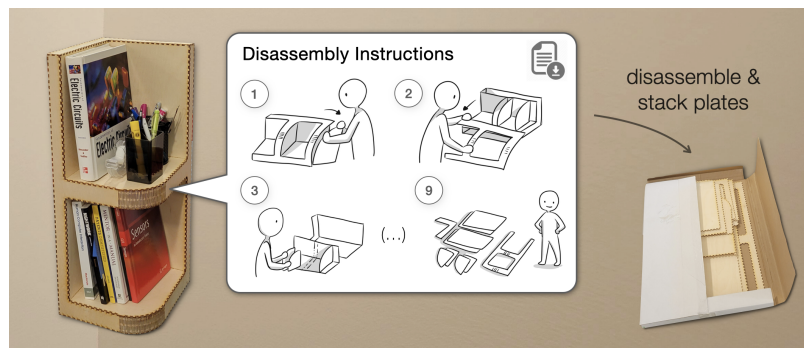
Figure 4-6: Disassembly instructions are linked to the shelf in case the user needs to take it apart for recycling or transport.
