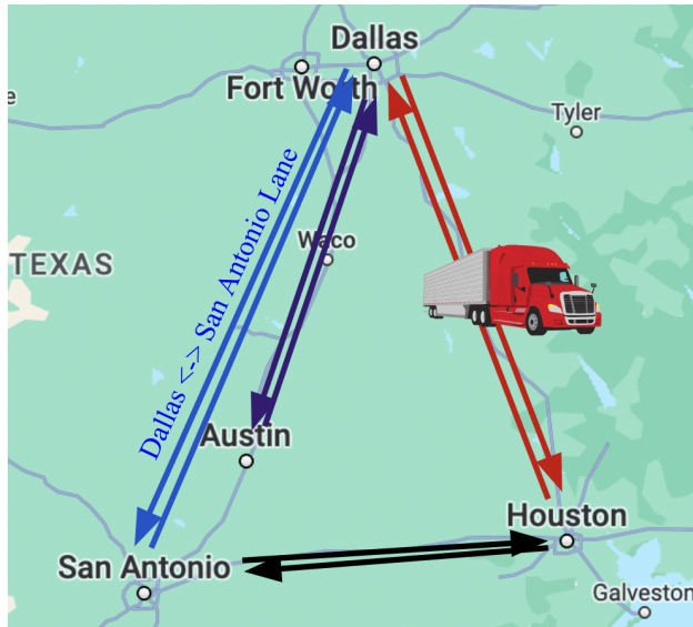
Figure 2.1: Visualization of the Texas Triangle, which is the network we use for the simulation. The arrows represent shipping lanes, such as the labeled Dallas to San Antonio lane and reverse. The truck logo illustrates how carriers drive between markets on lanes to pickup loads and deliver loads.
