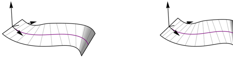
(b) Bending with prescribed torsion ( \tau(t) = 0 ). Successful bend (left) and premature termination with \varphi(t') = \frac{\pi}{2} (right).
