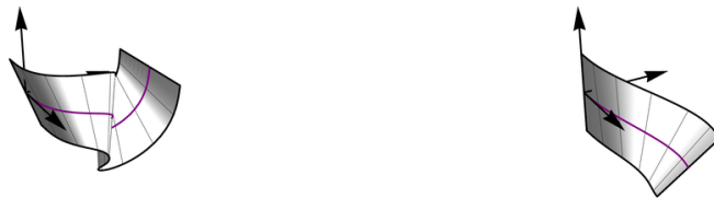
(d) Bending with prescribed curvature K(t) . Successful bend with K(\pi) = k(\pi) = 0 (left) and premature termination because |K(t')| < |k(t')| .
