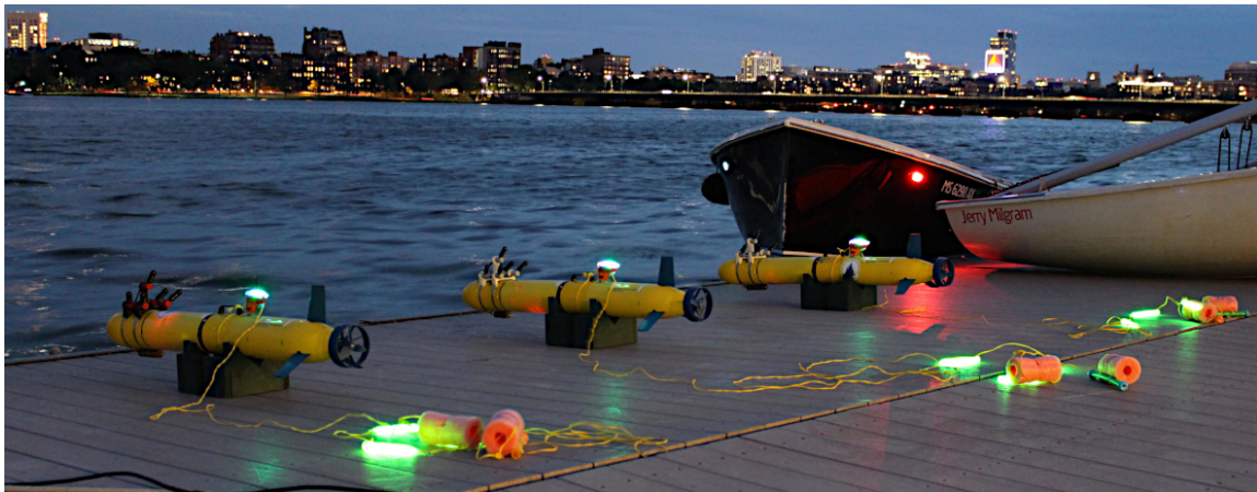
Figure 11. Photo of our Bluefin Robotics SandShark fleet during night operations in the Charles River with deployment from the MIT Sailing Pavilion and the Boston skyline in the background—strobe lights in the AUV masts and towed buoys with glow sticks provided a convenient way to monitor the AUVs when underway and underwater; the motorboat tied to the dock was used by two operators to reposition the OWTT-iUSBL acoustic beacon and to broadcast different commands to the fleet.
