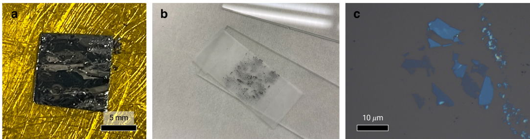
Figure 7-2: Mechanical exfoliation of SnSe crystal. (a) Photograph of bulk SnSe crystal, (a) Photograph of cleaved crystals on a scotch tape, (b) Optical microscopy image of exfoliated SnSe crystals of various thickness.
