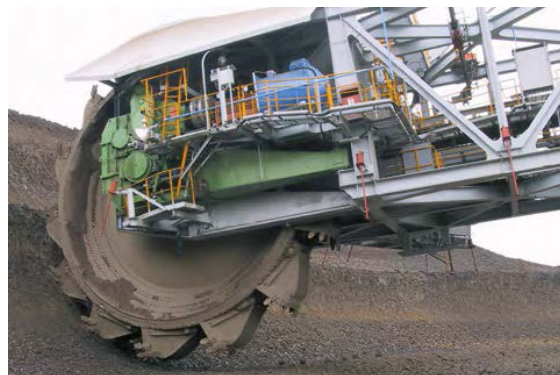
(e) Photo [6] of an excavator wheel driven through a hydrodynamic (fluid) coupling at an open-pit lignite mine.
