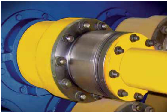
(c) Photo [4] of a coupling driving a leveler machine in a hot strip steel mill. The coupling does not slip or clutch on/off in normal operation, but incorporates anti-overload emergency disconnect functionality.
