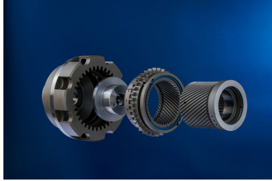
(b) Rendering [21] of an SSS (Synchro-Self-Shifting) Clutch, a type of overrunning clutch that transmits power in one rotational direction only. U.S. Naval vessels make extensive use of these couplings in various multiple-power-source Combined Marine Propulsion systems [22].
