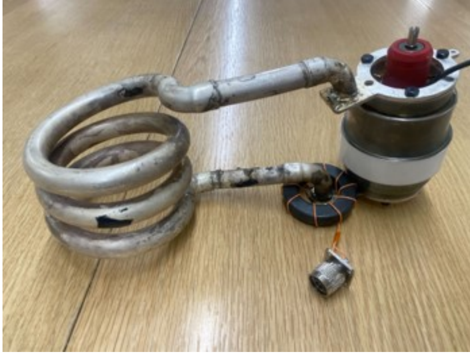
Figure 6-17: Air-core inductor series resonant network with a vacuum capacitor. Air-core specifications : 3 turns of 16 mm copper (wall thickness of 1 mm). Inner radius of the solenoid = 40 mm, pitch = 32 mm.
