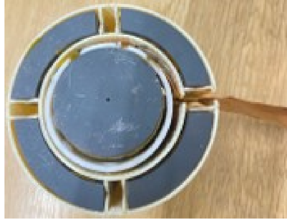
Figure 6-6: Top view of the center post, outer shell and copper winding
