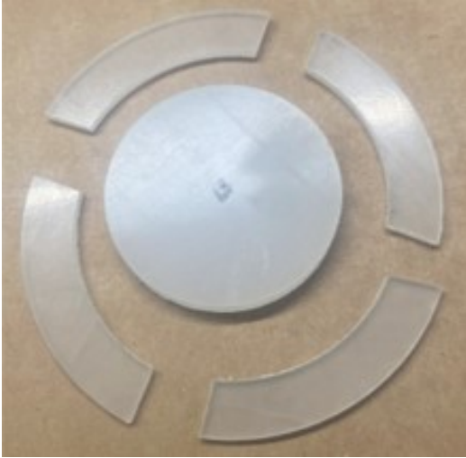
Figure 6-1: Polypropylene non-magnetic spacers cut using a waterjet cutter
