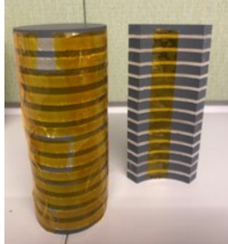
Figure 6-2: Center post and one fourth of the outer shell stacked using core pieces and spacer material, number of gaps = 13
