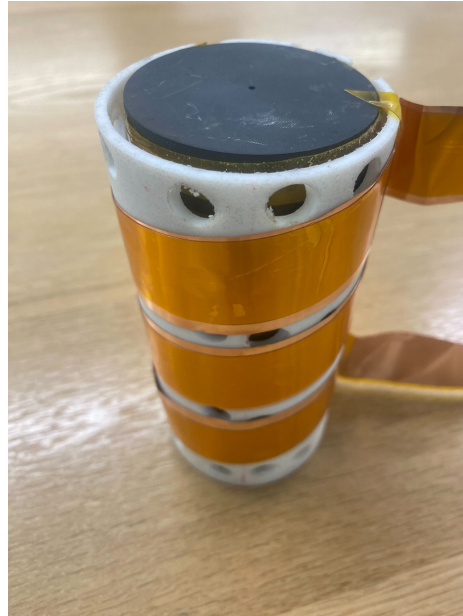
Figure 6-4: Cooper foil wrapped around center post through the PTFE support structure using double-sided polyimide tape
