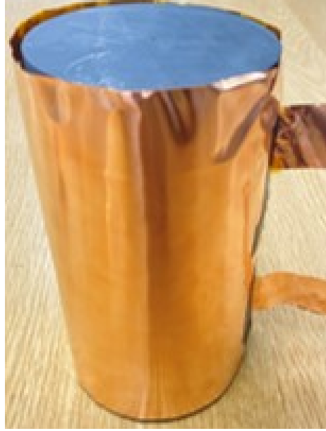
Figure 6-8: 75\mu\text{m} thick copper foil is wrapped around the structure to eliminate any fringing fields
