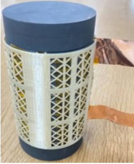
Figure 6-7: End caps enclosure the center post, winding and outer shell axially
