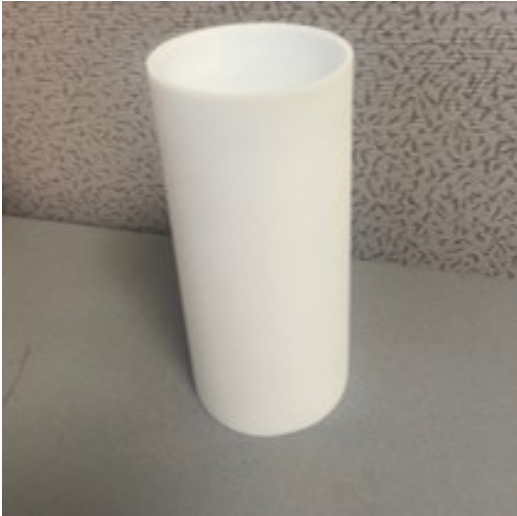
Figure 6-3: PTFE hollow cylinder machined to achieve desired height, outer and inner diameter
