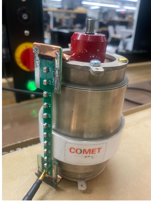
Figure 6-12: Calibration of the voltage divider ratio to estimate the total voltage across the vacuum capacitor
