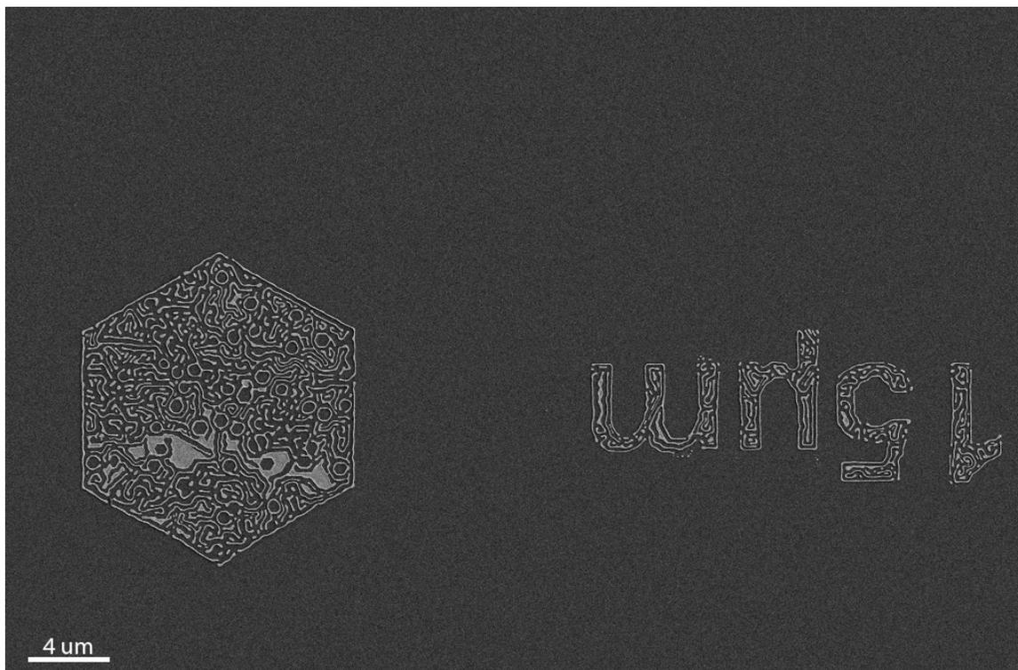
Figure C-19: A Ru patch which has been annealed for 45 minutes. The edges of the pattern are all  $30^\circ$  offset from stable  $\langle 11\bar{2}0 \rangle$  orientations. These edges have formed lines which are now in the process of breaking up.
