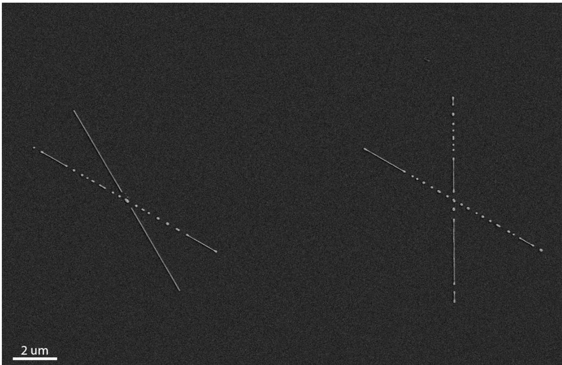
Figure C-18: Intersections of  $\sim 70$  nm-wide as-patterned lines. The left intersection contains one stable  $\langle 11\bar{2}0 \rangle$  line (oriented closer to vertical) and one unstable line. The right intersection is composed of two unstable lines.
