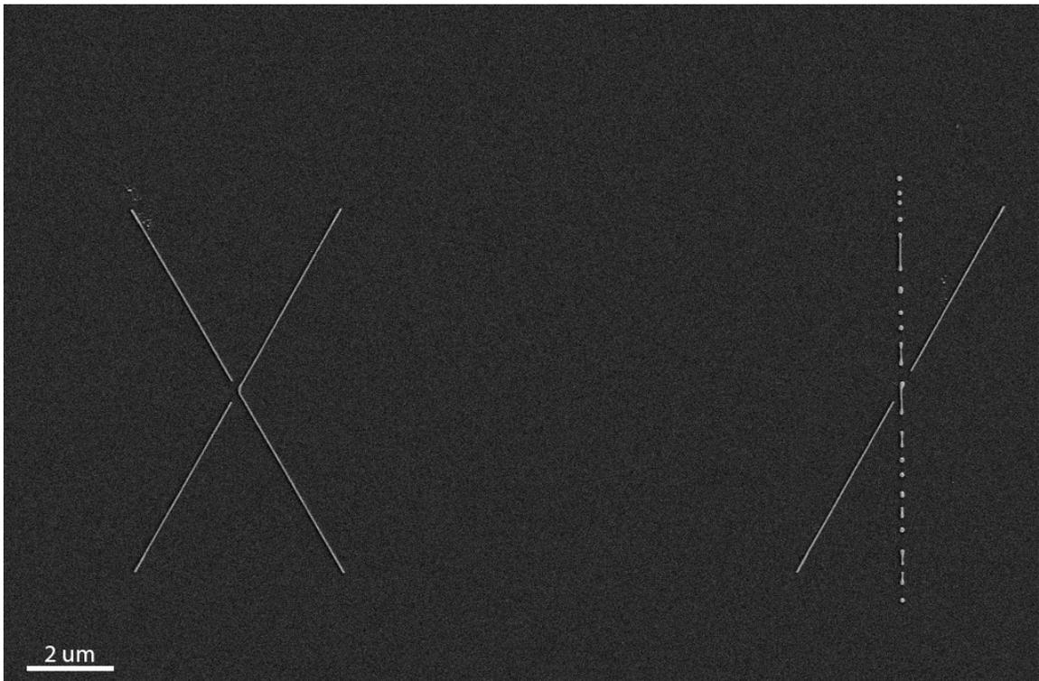
Figure C-16: Intersections of  $\sim 70$  nm-wide as-patterned lines. The left intersection is composed of two stable lines and has decomposed into 3 pieces: two lines and one sideways “V”. The right intersection contains unstable line (the vertical line) and one stable  $\langle 11\bar{2}0 \rangle$  line.
