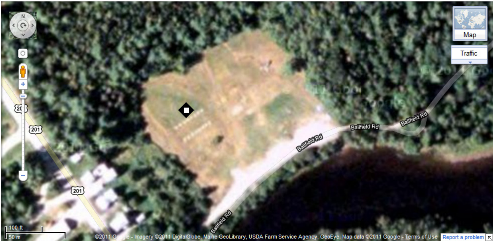
Figure 1. Location of EDGES antenna on Ballfield, Forks, ME. The active dipole was oriented along an azimuth of 30^\circ . (Horizon is limited by trees which have a maximum elevation of 25^\circ seen from the antenna.)
