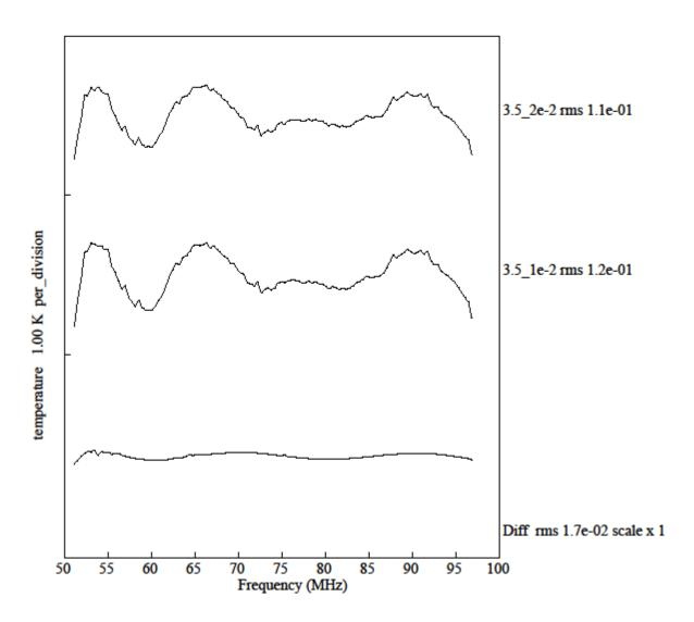
Figure 3. Difference between residuals using beam correction with different soil conductivity.
