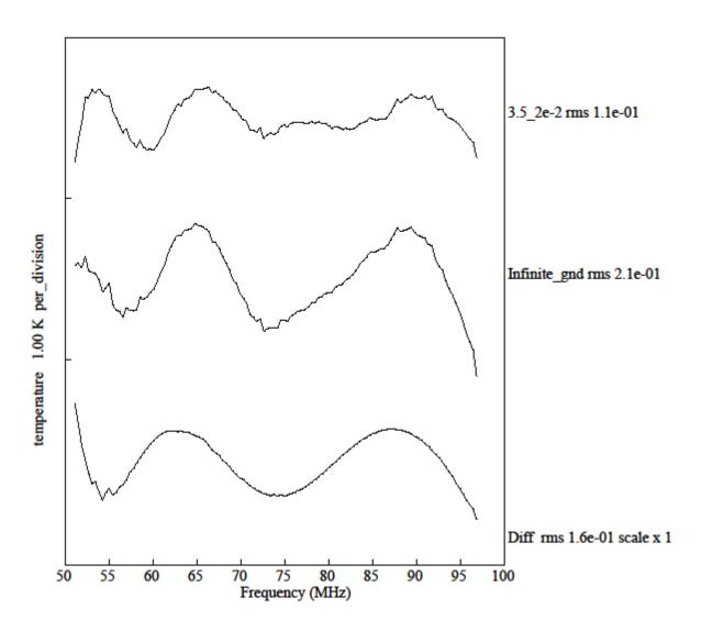
Figure 4. Difference between residuals using finite and infinite ground plane.
