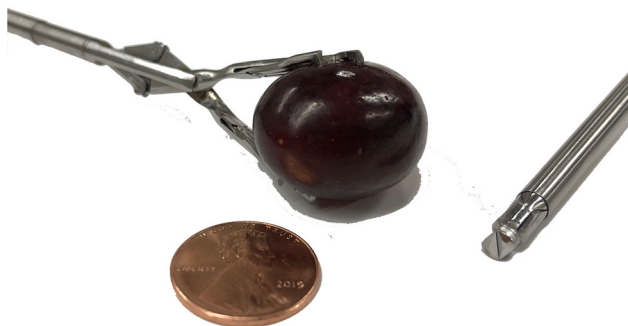
Fig. 8 Photograph of the two final prototypes. The unit on the left is open and grasping a grape. The unit on the right is in the collapsed state, as it would be for insertion through a trocar. A U.S. penny is shown for scale.
