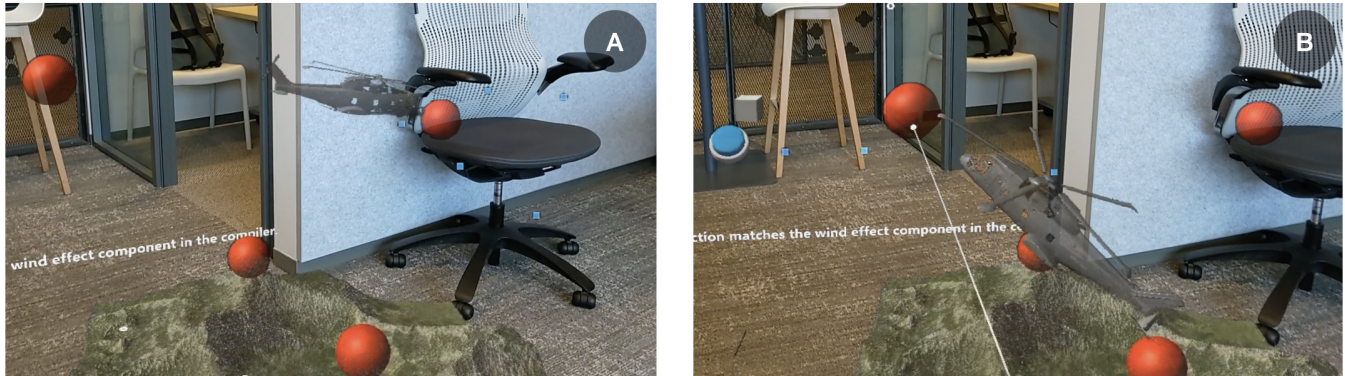
Figure 12: Simulated Rescue Plan . The HoloLens 2 displays the automated generation of a simulation of a rescue plan using our framework. The guide shows an interactable 3D terrain, helicopter, and simulated wind, allowing rescue workers to visualize the flight path under different weather conditions.
