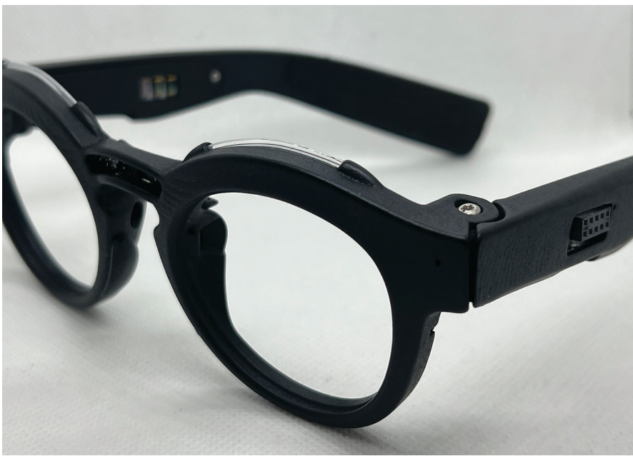
Figure 1. AirSpecs smart eyeglass device designed to measure environmental parameters and physiological parameters.
