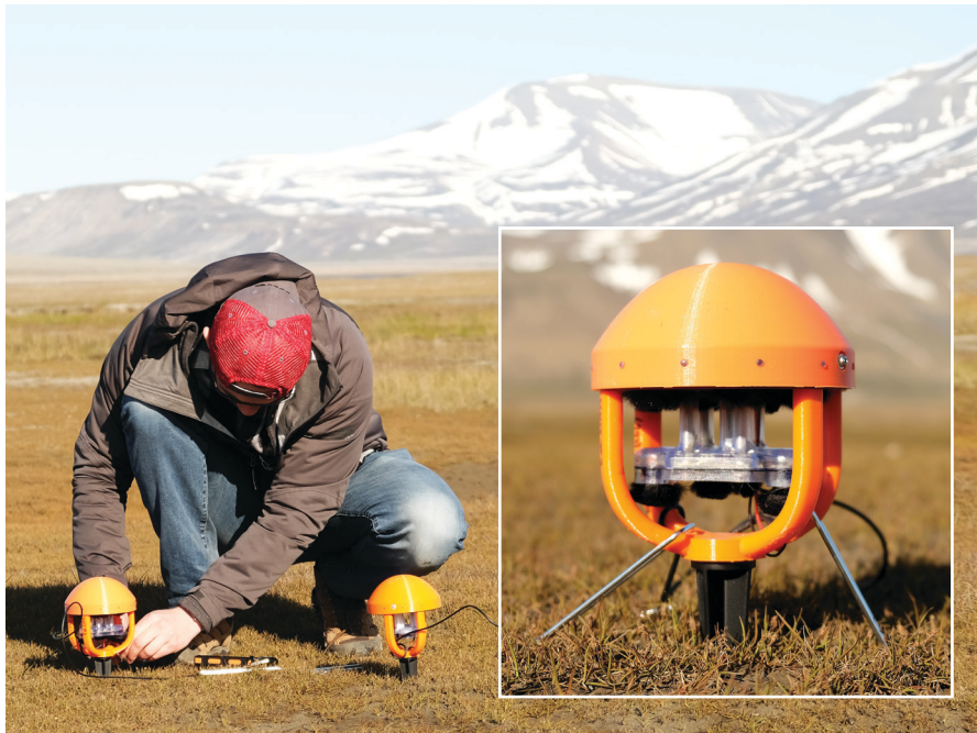
Figure 4. The SoundSHROOM microphone array devices deployed on Svalbard, a Norwegian archipelago in the Arctic Ocean, during the summer of 2023.
