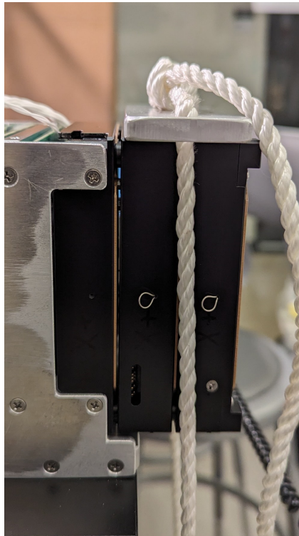
Figure 5.14: Picture of the 0.66 mm gap caused by the static load from -Y side.
