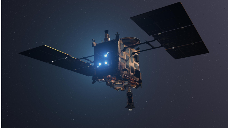
Figure 1.2: Hayabusa2 firing its solar-powered gridded ion thruster
