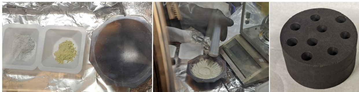
Figure 4.6 Electrolyte synthesis process in glove box (a) BaS and La 2 S 3 powders (b) mixing of these powders with FeS (c) Graphite pucker used to fill the 200 mg electrolyte mix in each drilled hole
