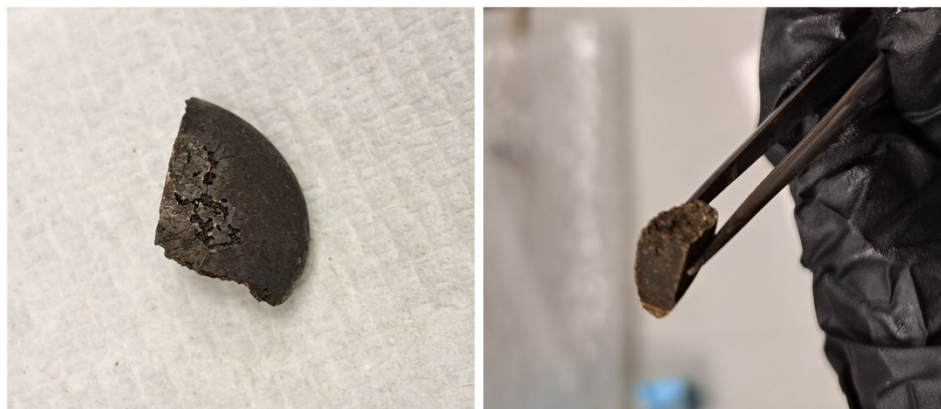
Figure A 2.3 Cross-section of the metallic pellet formed depicting (a) cracks on the surface mostly due to gas escaping (b) Fe-FeS phases on the cross-section
