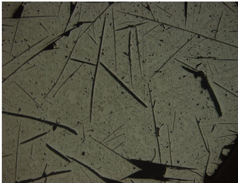
Figure A 2.6 Optical Micrograph of the Fe -C alloy metallic pellet produced as a result of the second VTT experiment
