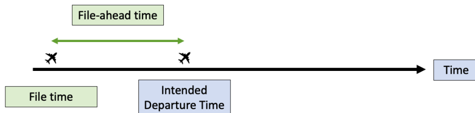
Figure 1.1: Representation of file-ahead time in relation to file time and intended departure time.
