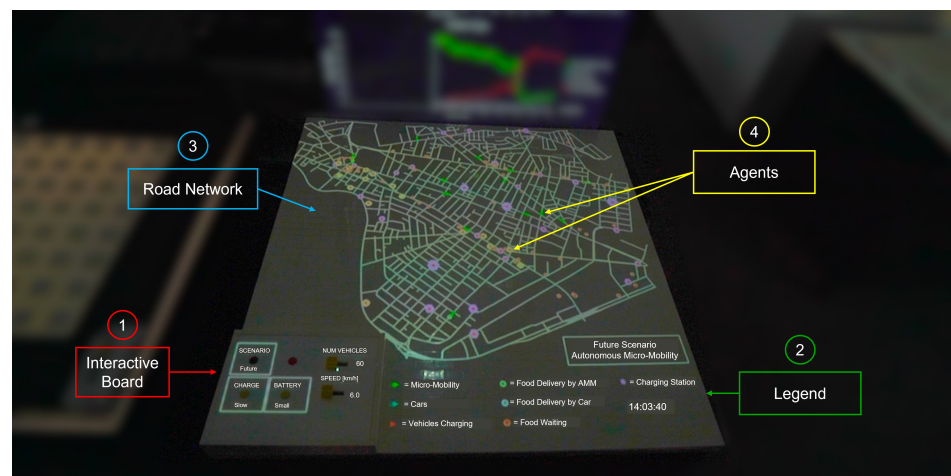
Figure 10. Interactive board (1—red), legend (2—green), road network (3—blue), and agents (4—yellow) displays that the user needs to analyze to generate insights.
