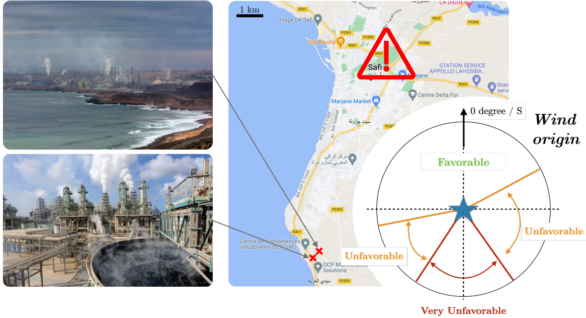
Figure 5.3: Wind direction and wind speed determine the dissemination of pollutants. Winds coming from the South with low speeds are the most dangerous conditions.
