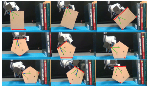
Fig. 10. Demonstrations: To test our framework, we regulate the system through a sequence of contact configurations. The measured robot wrench (blue) and the robot pose are used to estimate the friction constraints (green) and the contact locations and geometries (red). Top row: We execute the corner/corner pivoting primitive to move a rectangle from line contact with the ground to wall contact. Bottom row: We regulate a pentagon through sequence of contact geometry combinations.
