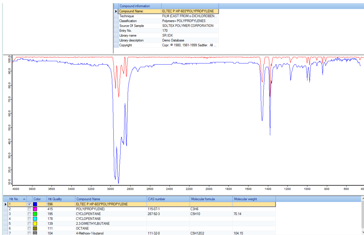
Figure A.10: FTIR spectra for polypropylene field sample 3
