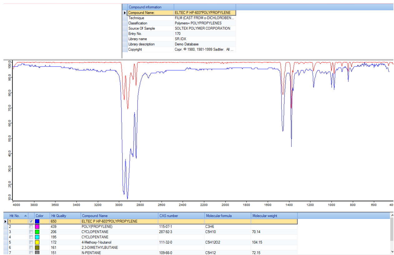
Figure A.9: FTIR spectra for polypropylene field sample 2
