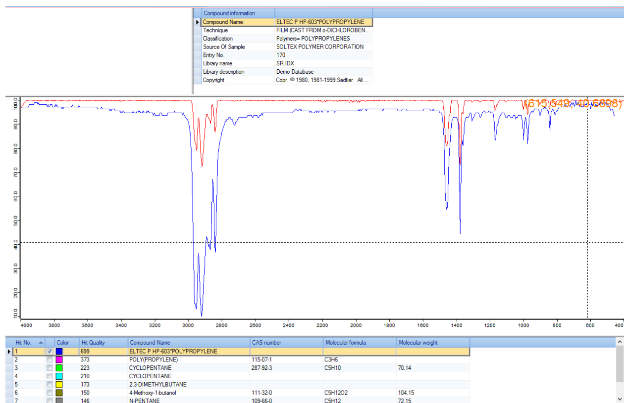
Figure A.12: FTIR spectra for polypropylene field sample 5
