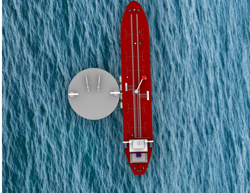
(a) Rendered Top Side View of Platform in STS Configuration
