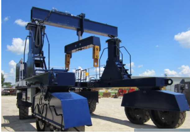
(a) Cask Transporter used to retrieve and place transport casks into the elevator.
