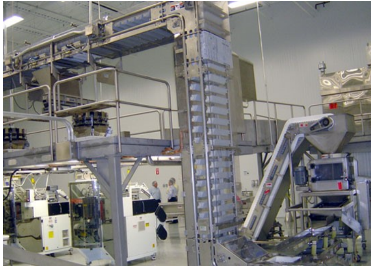
Figure 4.6: Heavy Duty Elevator Perspective View. [54]
