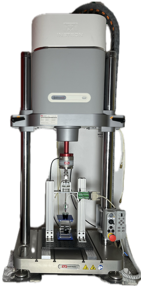
Figure 2-6: Nominal Instron Setup for VCCE Lab Experiments
