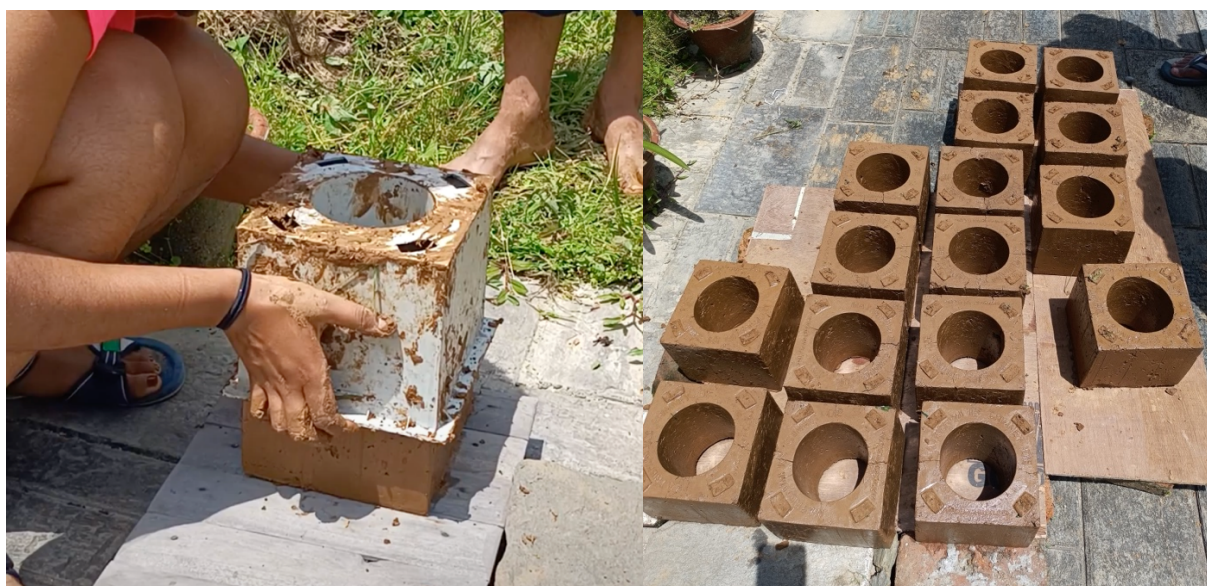
Figure 34: Chimney mold and drying chimney bricks
