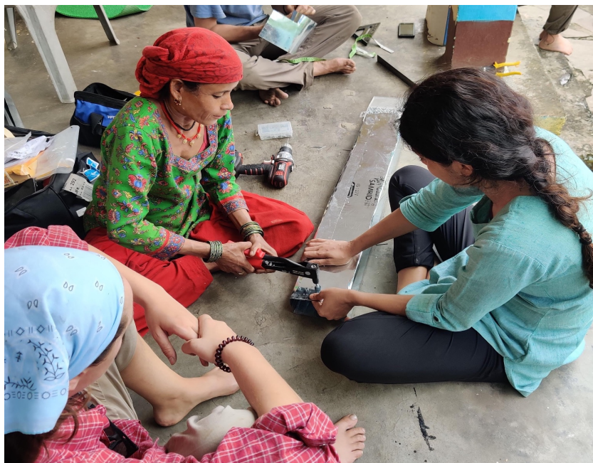
Figure 26: Left to right, Robyn Richmond, Samira, Sucheta Baliga fastening the chimney with rivets
