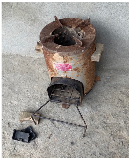
Figure 32: HotPoint stove, broken plastic handles pictured bottom left
