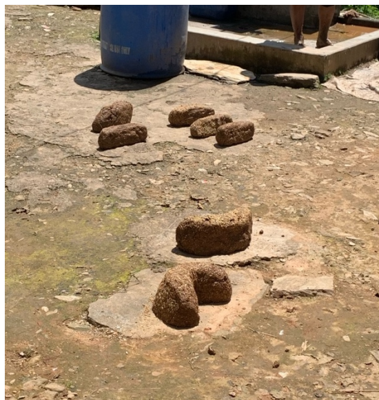
Figure 35: Sugar-salt-water-clay bricks for high temperature regions of the stove drying in the sun
