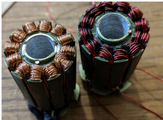
Figure 5.5: On the left this image shows the original as-purchased brushless motor rotor which has a low-torque-constant, low-resistance copper coil windings. On the right is the stator after being hand-rewound to increase its torque constant. A higher torque constant allows for reasonable battery powered operation with the low currents available to the brushless motor controller circuit board. Intuitively the thinner the wire, the higher the torque constant, but after some measurement it was discovered that the original windings have 6-8 fine wires that are all in parallel with each other. This likely allows for a better packing density, and potentially a higher surface area to volume ratio for cooling.
