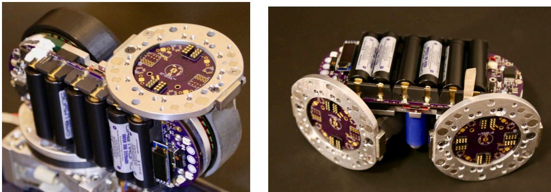
Figure 6.12: Before designing Belty a similar robot with direct-drive actuators was built and tested, named Flippy. There are many favorable characteristics of direct-drive actuators for assembly robot tasks including mechanical simplicity and high bandwidth control. However, the lower maximum torque and the lack of inherent damping made this prototype too difficult to safely operate given the maturity of the electrical system on the robot.
