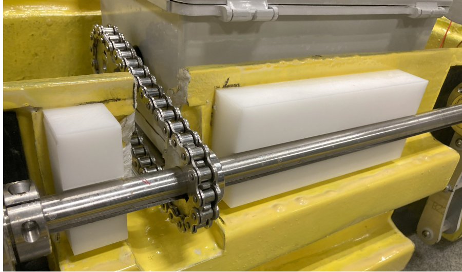
Figure 6.20: The arm motor, chain, drive shaft, and support bearings.
