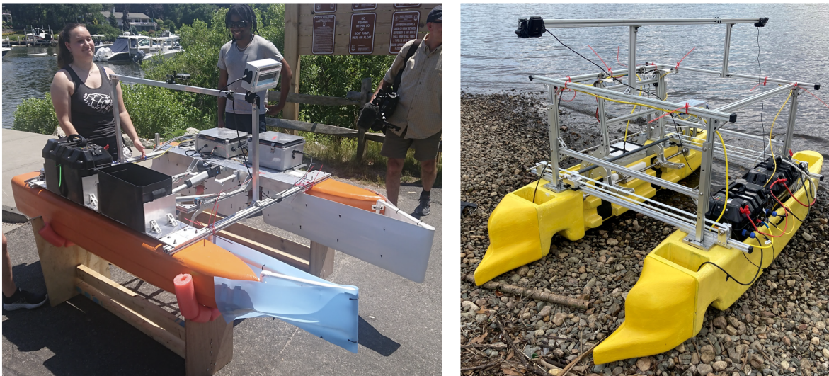
Figure 4.1: The hulls of the V1 (left) and V2 (right) Oystermarans. The V1 vehicle has additional guides attached to its bow which allowed it to fit into the field and were added during its testing and redesign process. The bows of V2 were interchangeable, the "combination" nose, the final one developed, is shown.
