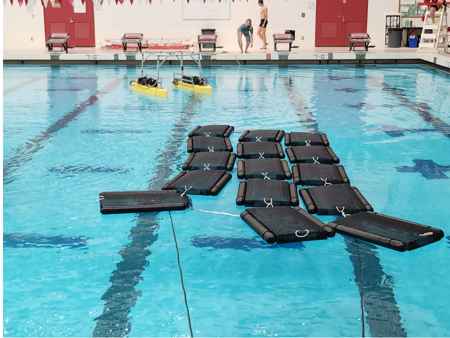
Figure 5.1: The unweighted oyster array setup. The front holding pole and rope are both visible in the front, with the V2 Oystermaran on the left.
