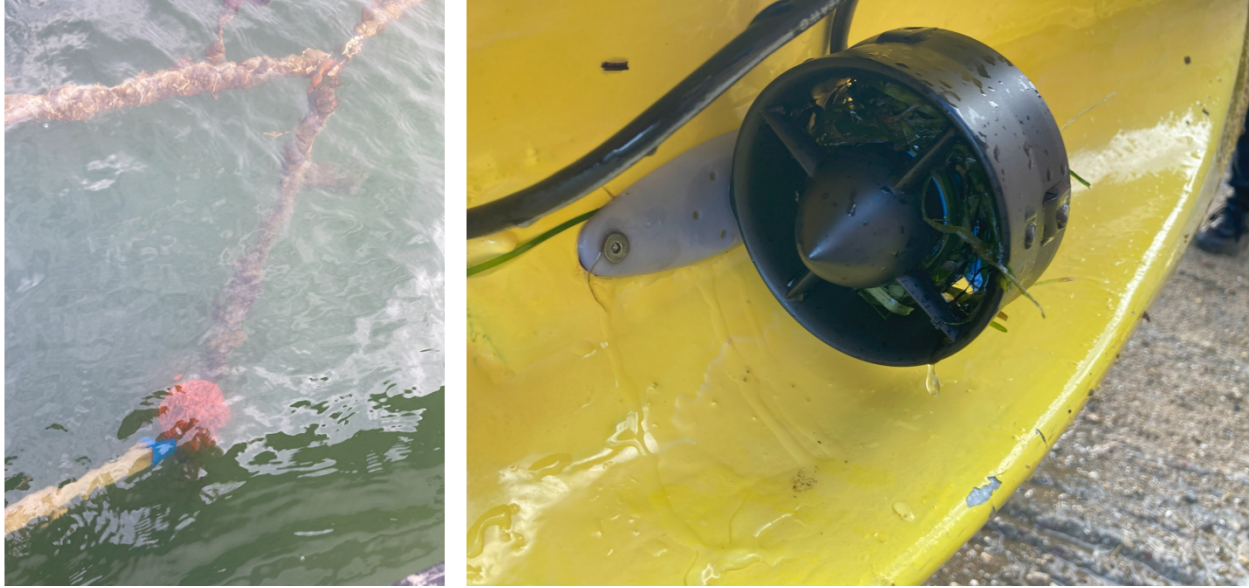
Figure 5.12: The thrusters experienced significant biofouling, much of which came from entering the array over the frame shown on the left. On the right, a rear thruster filled with seaweed.
