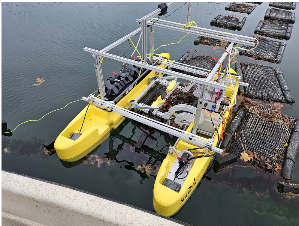
Figure 7.1: The vehicle and flipping mechanism during Field Test II. Note the mechanism is slightly raised, though it was unable to travel higher than this.
