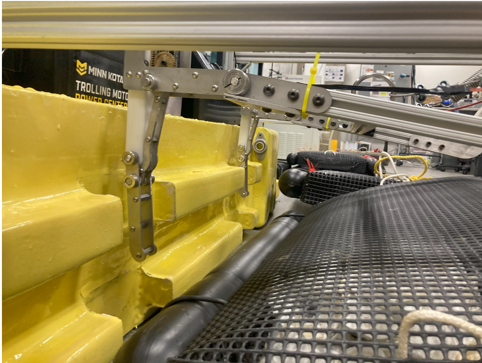
Figure 7.10: The open claws sliding back into their insets around the basket. the arm is low enough that the basket is already laying on the floor after being flipped.
