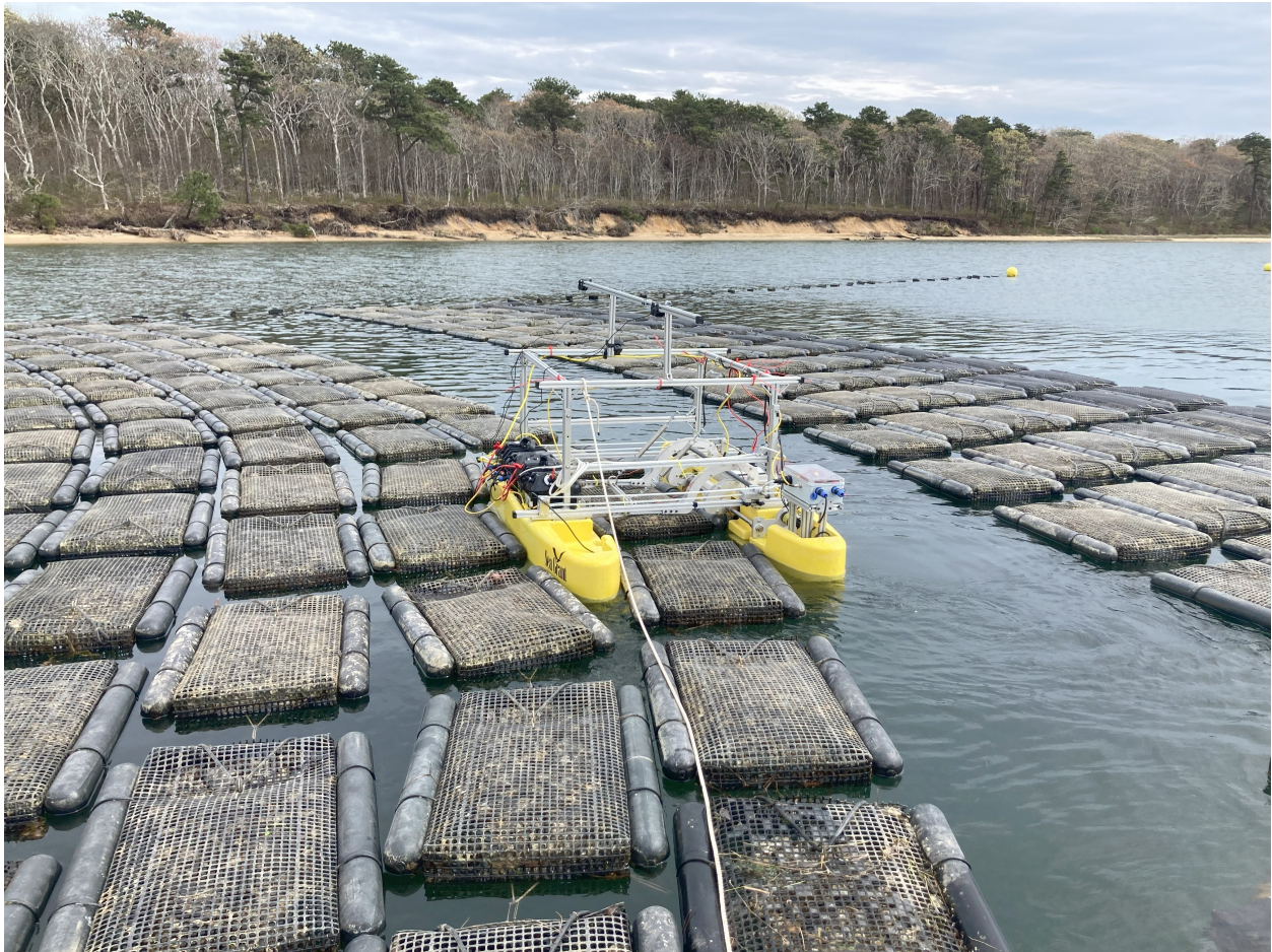
Figure 3.2: The Oystermaran V2 in the field with all mechanical systems complete.
