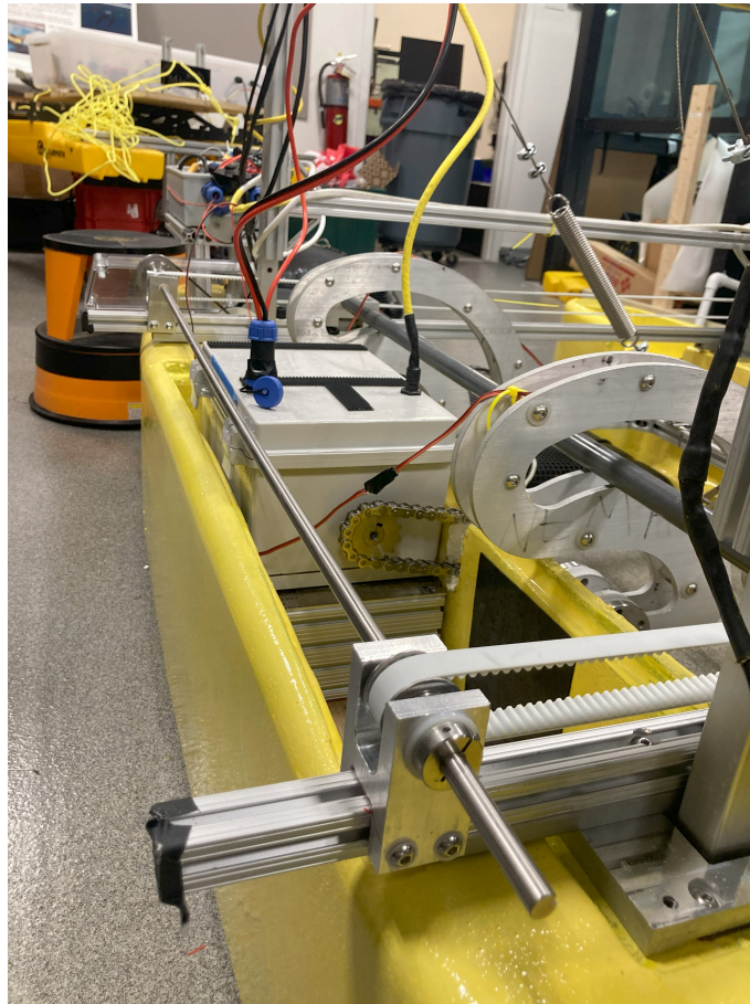
Figure 6.22: The slider pulleys mounted on their drive shaft. The drive shaft is keyed, with keys constraining the rotational motion and shaft collars constraining linear motion along the shaft.
