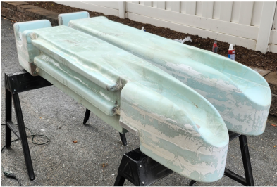
3. Fiberglass applied and beginning of sanding/filling
