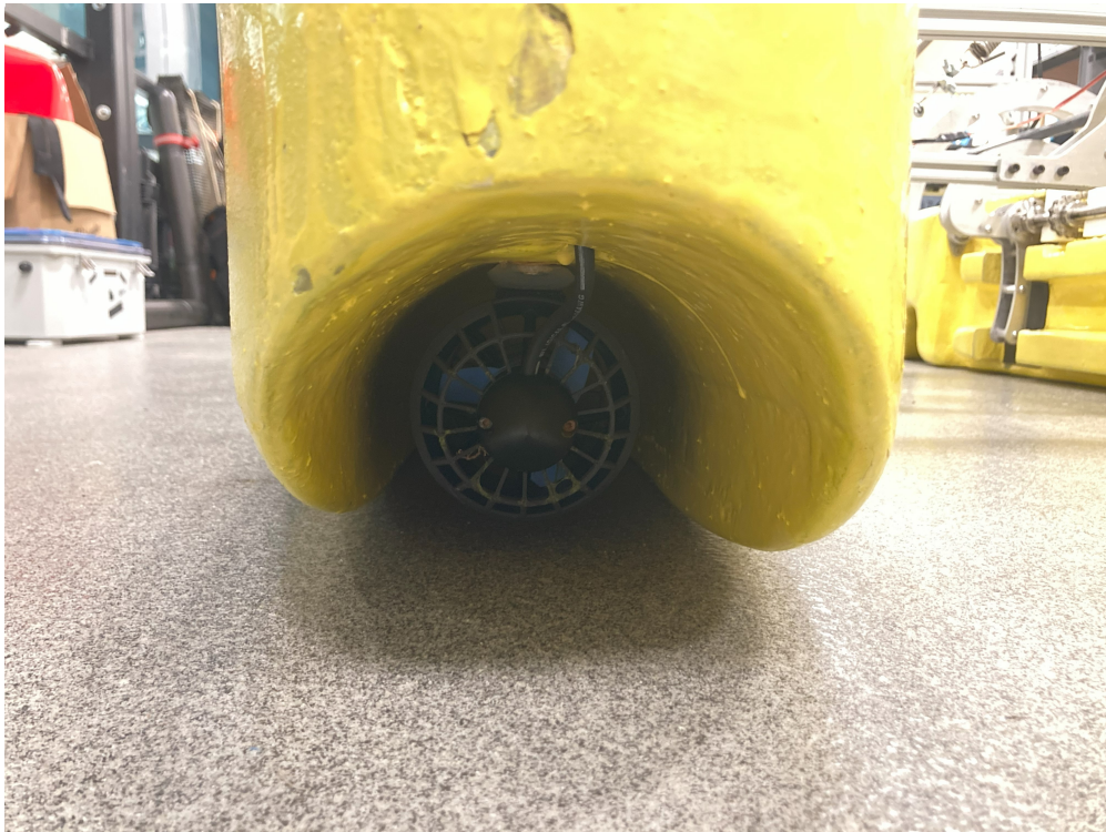
Figure 5.16: A fully protected rear thruster. Visible are both the surrounding shape of the thruster channel as well as the thruster cage. Slight discoloration can be seen from testing, but no biofouling became entangled with any of the thrusters.
