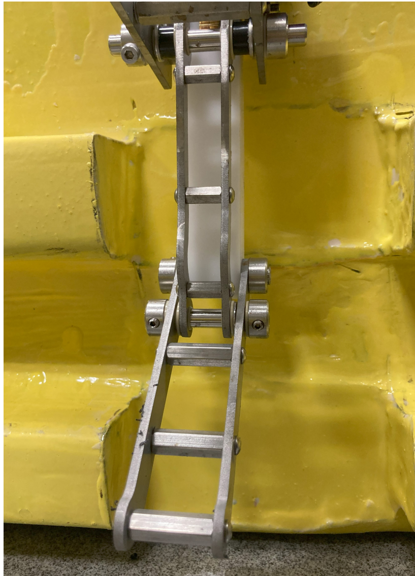
Figure 6.12: The inside of the claw, where the spacers which constrain the links to rotary motion can be seen along the shafts next to the guiding link.
