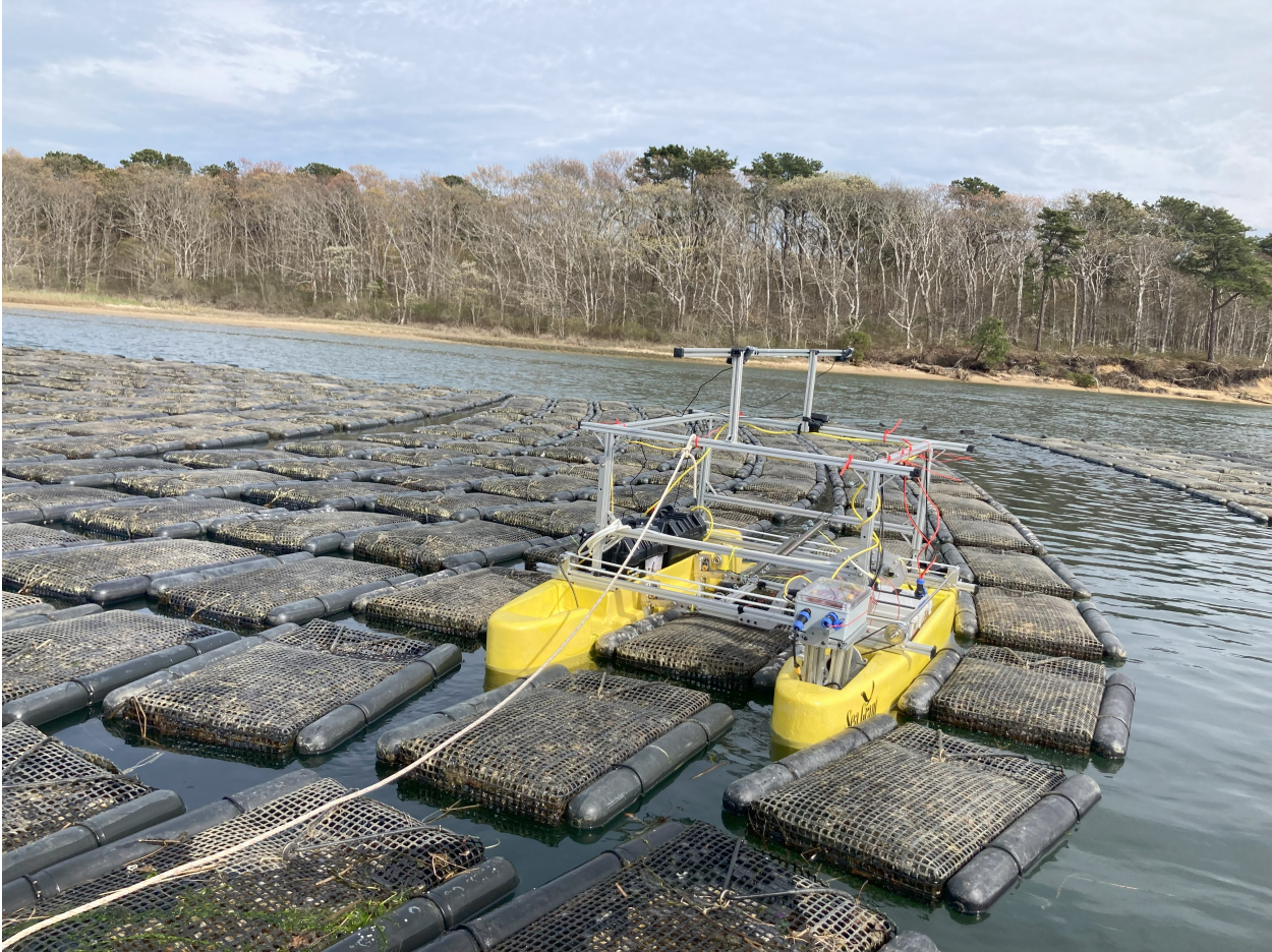
Figure 7.12: The Oystermaran in the array. Maneuvering was generally successful, though still required some effort to enter between the rows.
