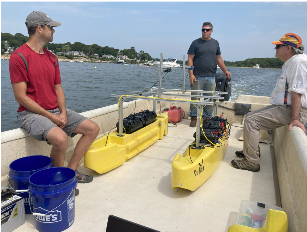
Figure 5.9: Transporting Flippy to the oyster farm in a work boat. Note the adjustable frame and lack of flipping mechanism.
