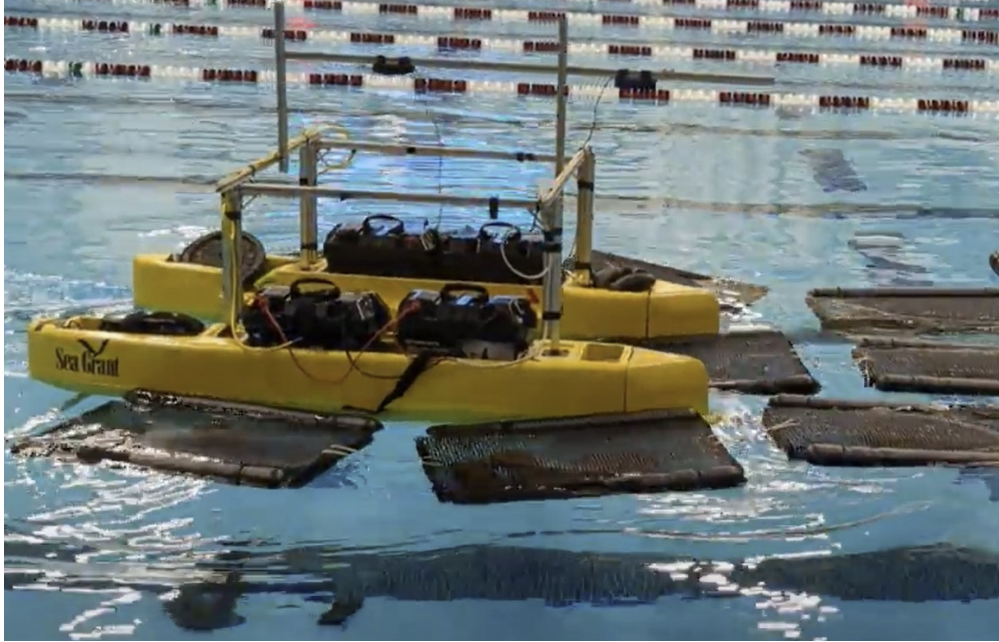
Figure 5.7: The hulls with the anti-rising nose traveling through the weighted array. As the pointed portion of the nose is below the water, little of can be seen in this image. An underwater photograph is displayed in Fig. 5.8
