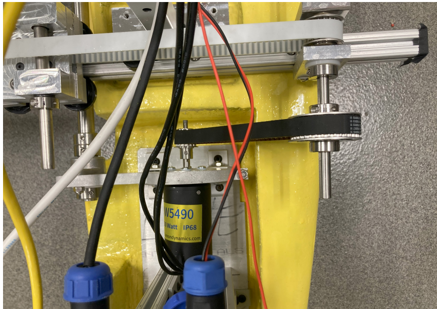
Figure 6.26: The motor mount, which allows for tensioning of the drive belt. It also mounts the arm drive shaft, which can be noticed on the left.
