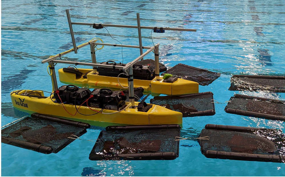
Figure 5.6: Here, while using the asymmetric guide nose the port hull can be seen pushing the central basket into position while the starboard hull pushes the exterior row away.
