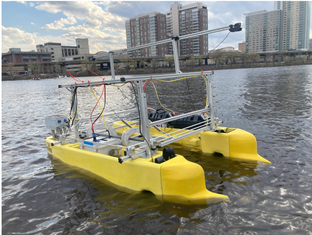
Figure 5.17: During testing of where the waterline needs to be on the vehicle for it to travel over the baskets while still being able to grab and flip them. Notice how the vehicle is higher in the water than usual.
