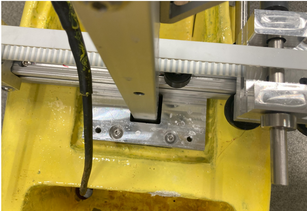
Figure 6.23: The rail mounts for the slider beams, which mount to the hulls around the frame posts. In this image, the slider is mounted to the inner mounting location with the tapped holes for the outer configuration visible.
