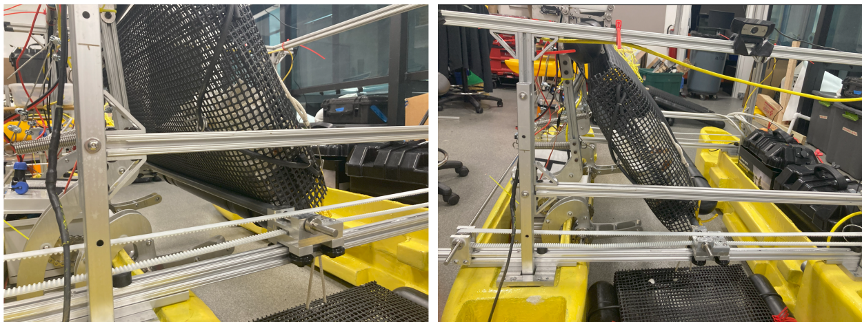
Figure 7.6: Left: The underside of the slider just after removing the basket from the basket rests. Right: The slider halfway across its rail, the end of the pushing step
