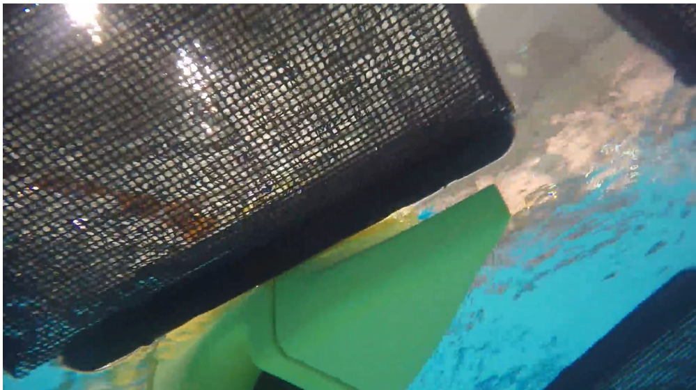
Figure 5.8: The anti-rising nose passing underneath the the edge of a basket.
