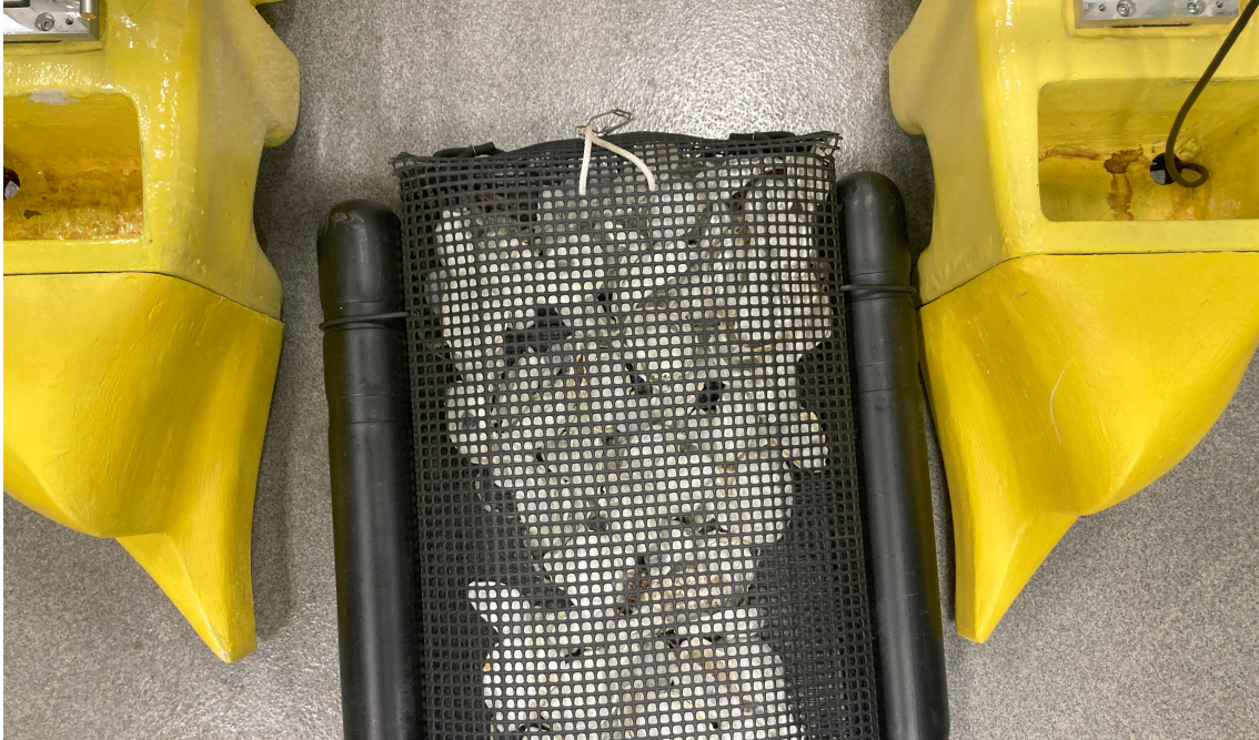
Figure 5.14: The combination nose shown in the lab surrounding an oyster basket. Note the points of the noses coming close to the baskets to reduce the spacing between them.
