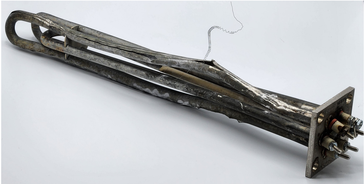
Figure 4.18: Boost heater from the dishwasher. Note the filament wires sticking out. Corrosion did the damage to the heater – according to the technicians, removal did virtually no damage to it.
