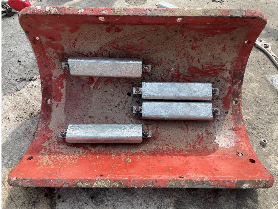
Figure 1.4: New zinc sacrificial anodes.
