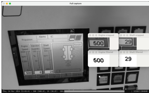
Figure 3.19: Screenshot of the OCR script transcribing values from the engine control unit.
