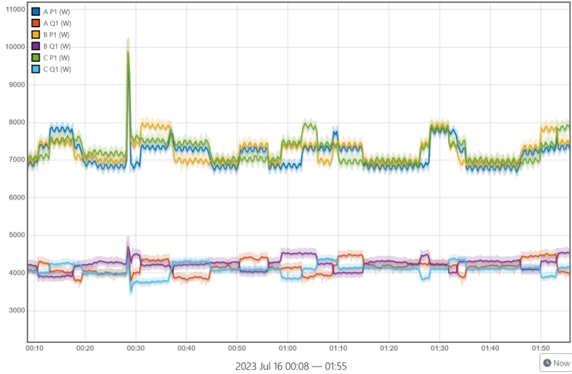
Figure 4.7: Signature from the HVAC main control panel, showing miscellaneous equipment and harmonic distortion from the HVAC control systems.
