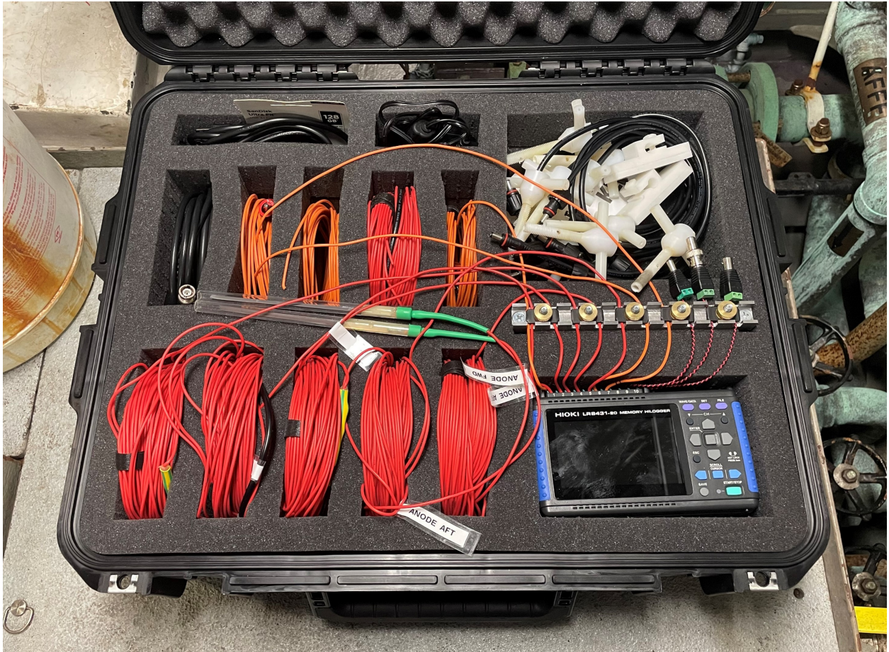
Figure 2.15: The data acquisition kit used in the Margaret Norvell experiment.
