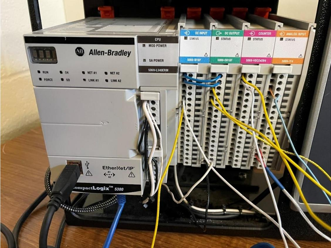
Figure 5.2. Allen Bradley 5380 Compact Logix Modules.
