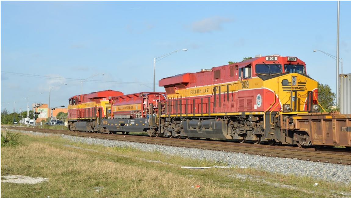
Figure 3-14: Florida East Coast Railway Locomotives and LNG Tender Car [43]
