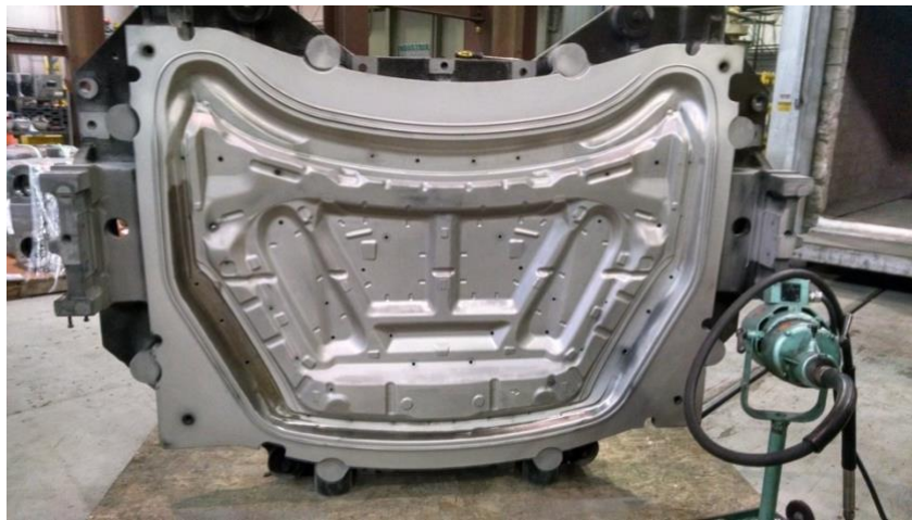
Figure 2-2: Image of Stamping Die for a Hood (Enhancing Durability of Automotive Stamping Dies with Plasma Nitriding, n.d.)
