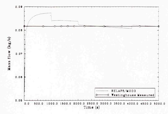
Figure 5. Mass flow rate (kg/s) vs. time (s) in the hot leg for test SG-S2. This problem was restarted every 1000 s with different  $k_{loss}$  values in order to effect convergence with experimentally measured results.
