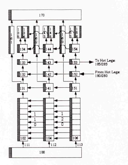
Figure 2. The nodalization diagram of the RPV is shown. Note the three channel core and the multi-directional flow volumes in the upper plenum. These multi-directional flow volumes enable natural circulation to occur throughout the RPV. Shaded areas represent metal structures. The arrows indicate the positive flow direction, not necessarily the actual direction of flow.
