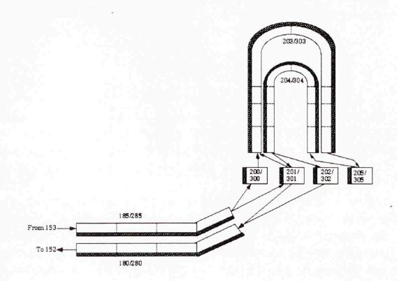
Figure 4. The nodalization diagram of the hot leg is shown. This is a split, countercurrent flow hot leg model. However, the split hot leg shown does not represent accurately the sloped portion of the hot leg. There is no pressurizer modeled because the Westinghouse apparatus did not have one. Again, shaded areas represent metal structures.
