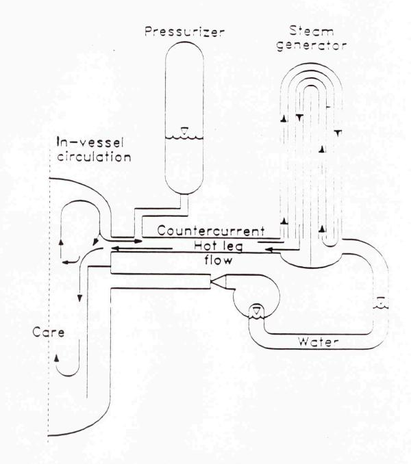
Figure 1. Natural Circulation flow pattern both in-vessel and ex-vessel during some severe accidents. Flow rises from the core into the upper plenum, where it splits to flow into the hot legs and back down into the core. Hot leg countercurrent flow arises, as does steam generator tube flow.
