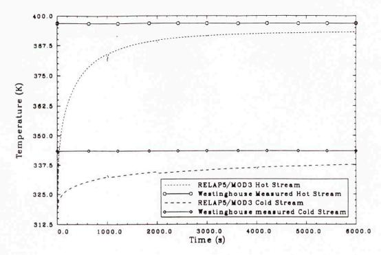
T vs. Time in Flow Streams of Hot Leg, Test SGS1
