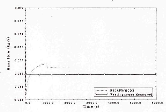
Mass Flow vs. Time in Hot Leg, Test SGS1
