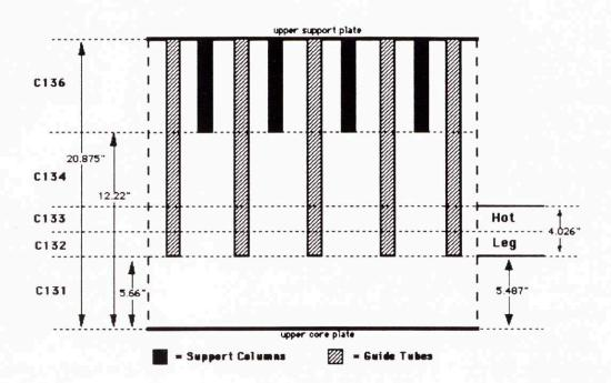
Figure 3. Schematic view of upper plenum geometry in the Westinghouse experimental apparatus, leading to considerations in devising the nodalization of the upper plenum for the RELAP5/MOD3 model. Note the divisions at heights level with the endpoints of certain structures in the upper plenum, such as the hot leg pipe level, the support column level, etc.
