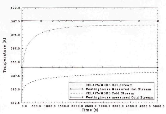
T vs. Time in Flow Streams of Hot Leg, Test SGS2
