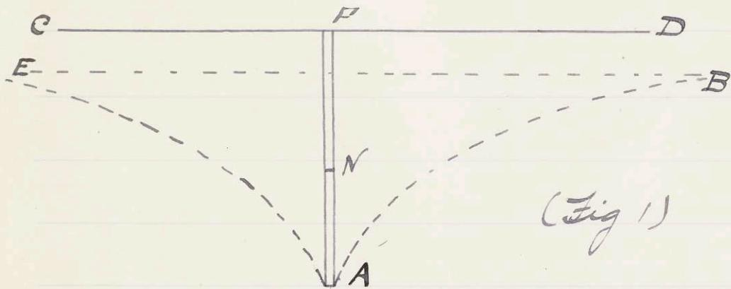
of the ground, and EB the level of the water table. Now if water be pumped from the well FA, the surface of saturation will take some curve as AB. The shape of this curve and the distance it extends in the direction EB before it becomes
