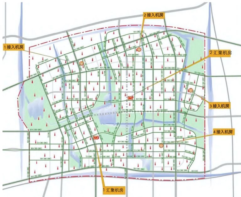
Figure 30. Plan of Rongdong District showing distribution of “edge computing macro stations” and sensing poles (Liu et al 2022)
