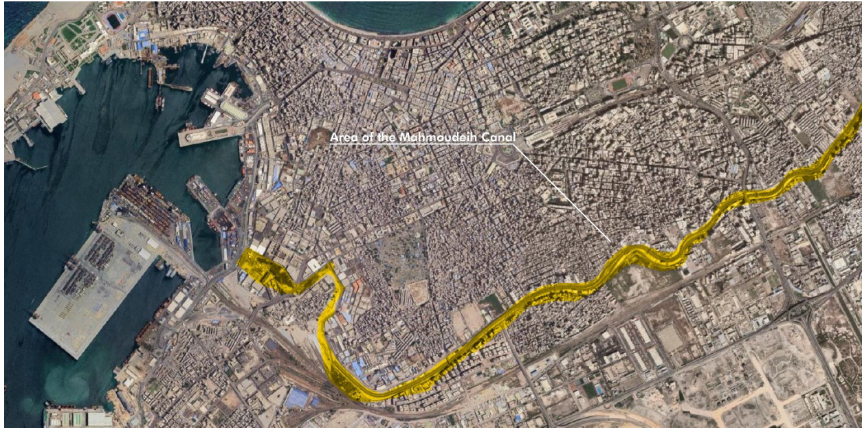
Fig. 21 – Satellite image of contemporary Alexandria with the sinuous shape of the elevated highway, Elshohada Square Rd, inherited from the water channel of Mahmoudieh Canal. Source: author.
