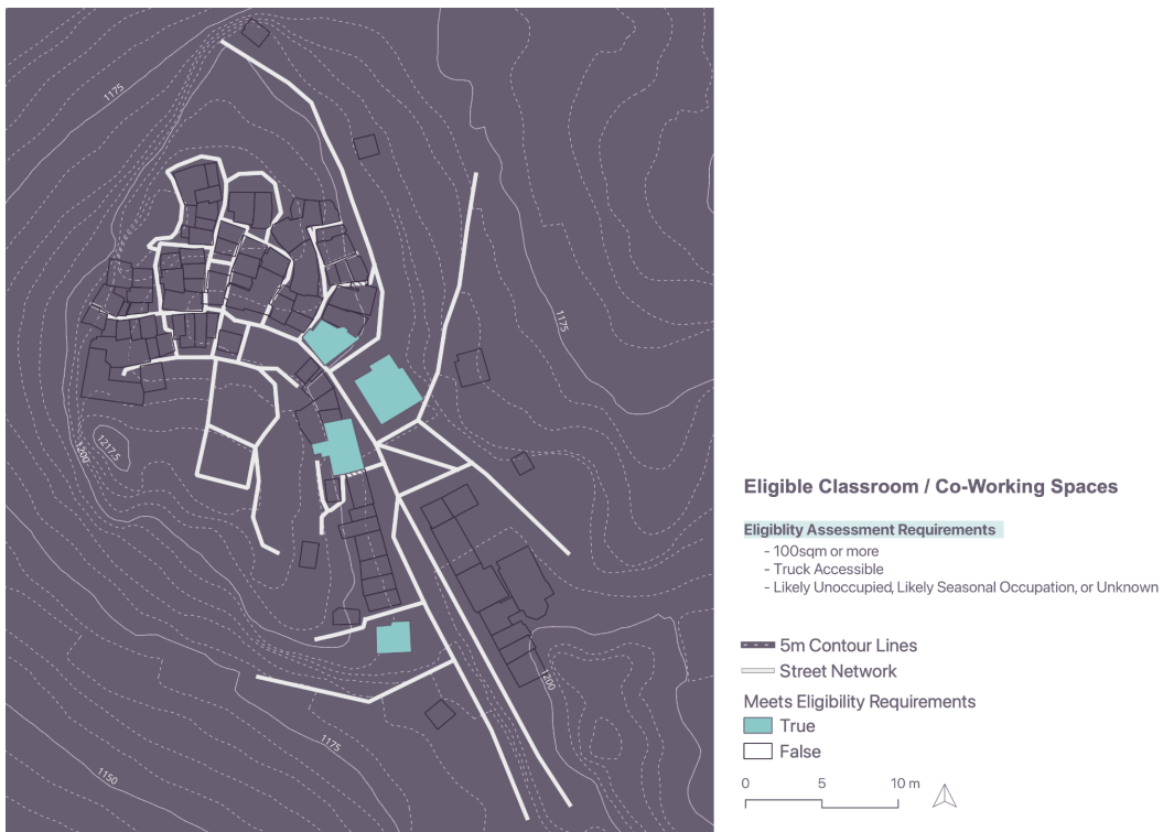
Figure 30: Map of eligible working spaces for Guadagnolo. This map depicts the buildings that meet all three eligibility criteria to be leveraged as working spaces for either reuse scenario.
