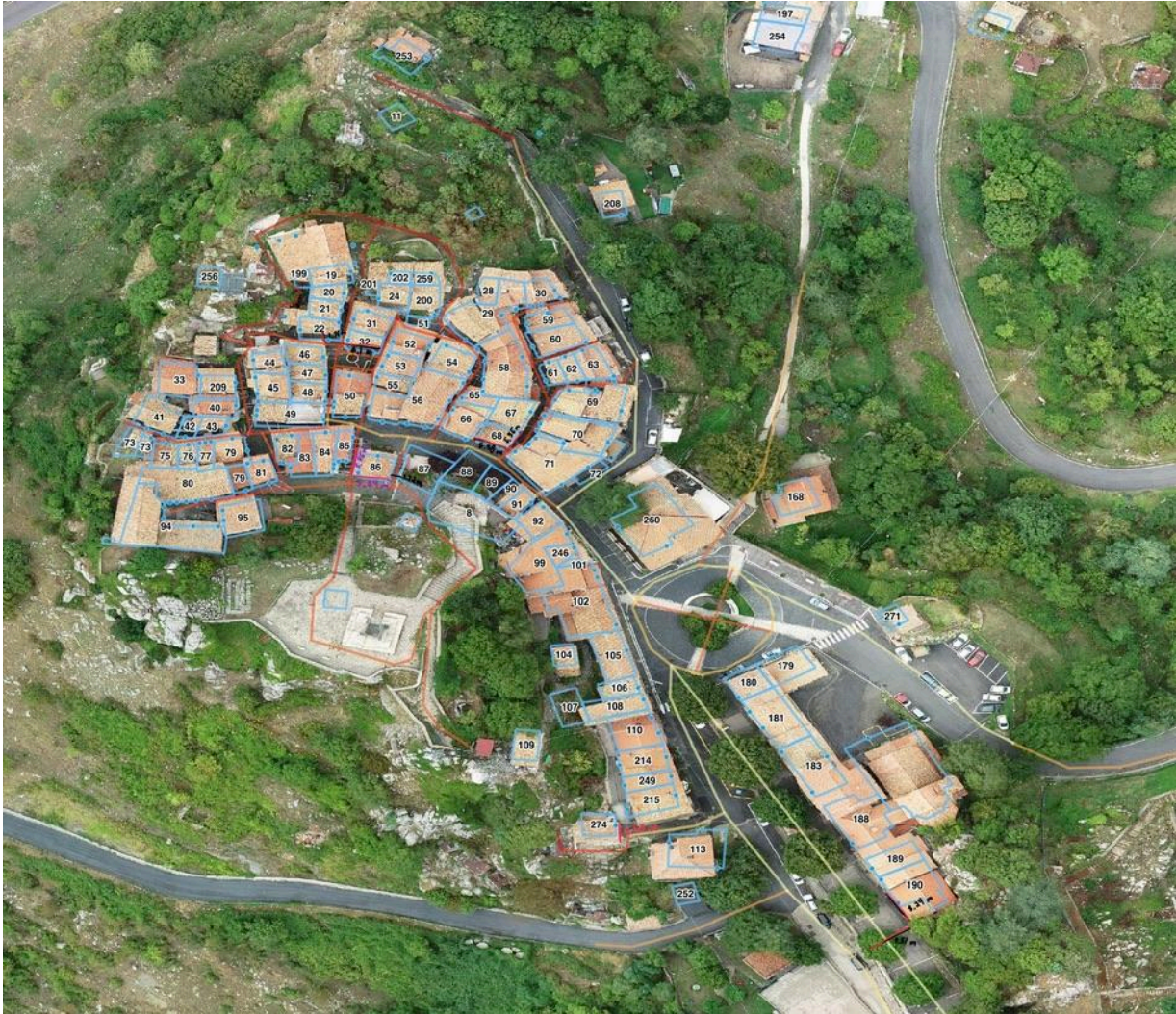
Map of Guadagnolo overrated with the provided municipal map. Plat in the municipal map and existing buildings in the orthophoto did not align which is why a re-tracing of each lot using the orthophoto was needed.
