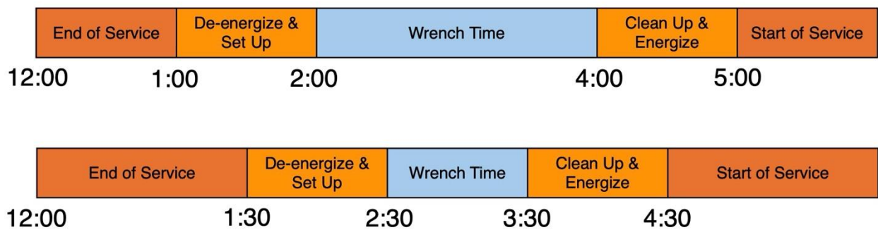
Figure 19: Graphic showing hypothetical overnight maintenance window under a normal schedule (top) and a one hour extended schedule (bottom) showing total wrench time is cut in half.
