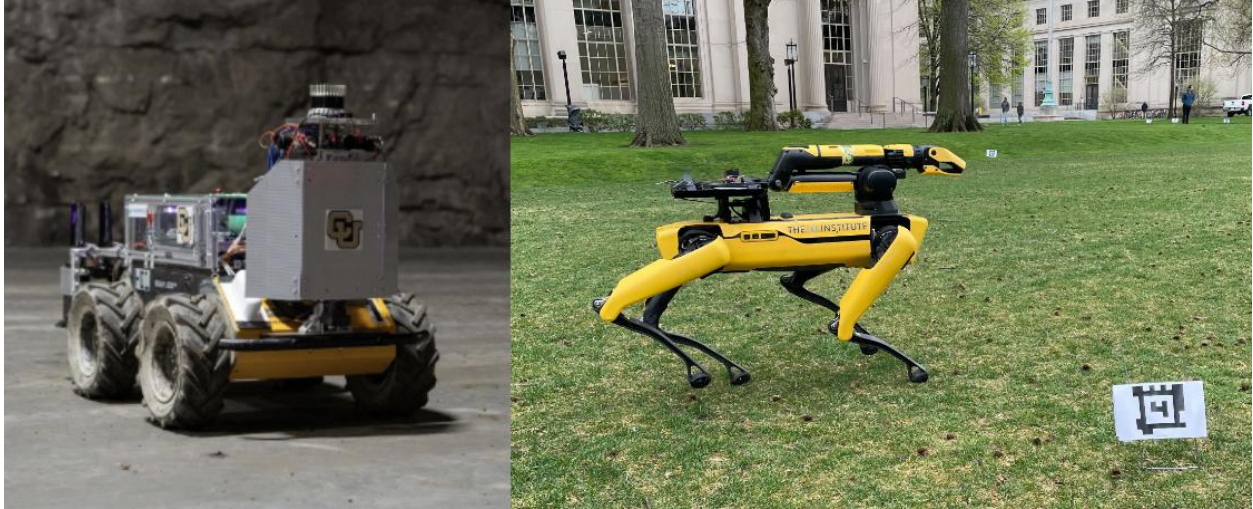
Figure 1.6: Mobile systems like the Husky [7] and Spot [11] often have limited compute due to payload and power supply constraints.
