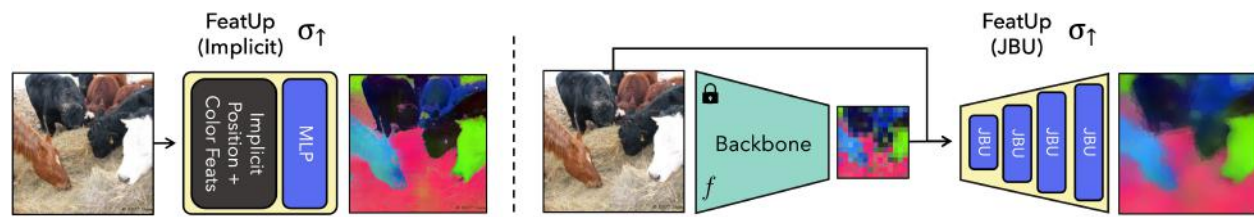
Figure 2.7: Our Implicit version of FeatUp learns an implicit network to upsample a single image’s features. Our JBU FeatUp learns a stack of JBUs that learns to quickly upsample features from a large image corpus.
