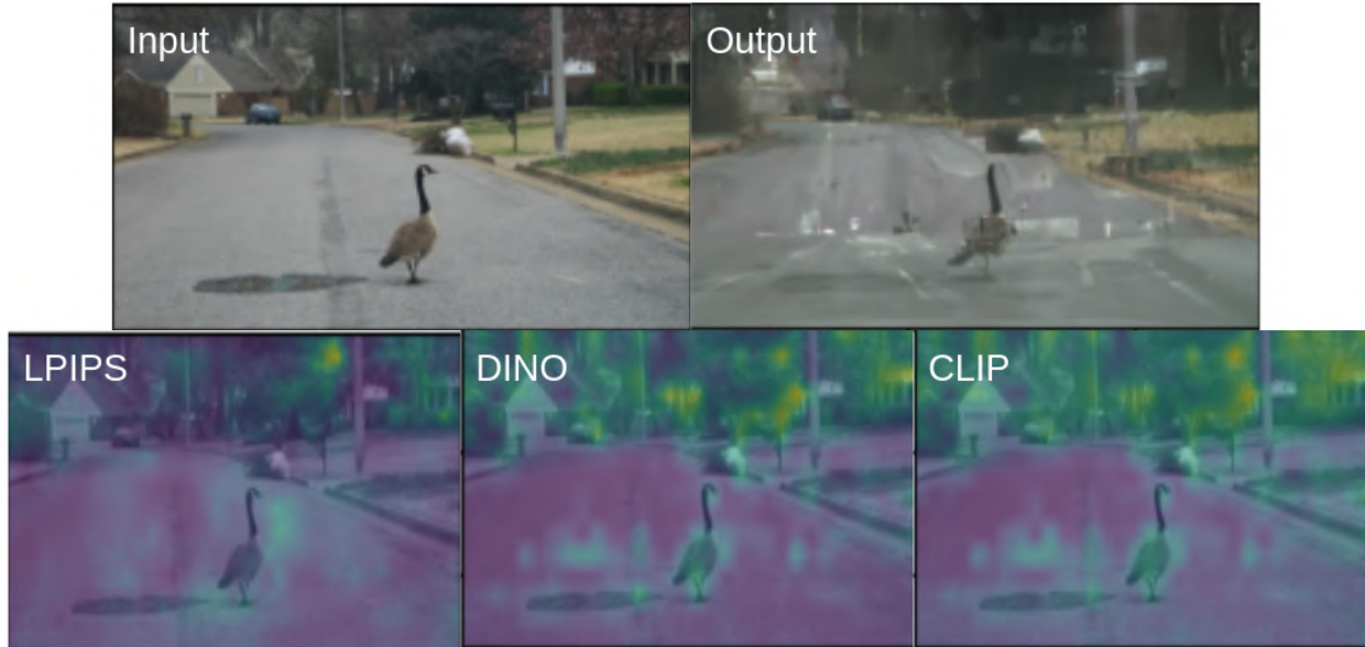
Figure 4.2: We tried guiding the diffusion model using the LPIPS perceptual similarity metric. This yielded the output at top-right, which clearly still had something ‘goose-y’ in the foreground. We then computed the LPIPS, DINO-based, and CLIP-based differences between input and output, and saw that the majority of perceptual changes had actually occurred in the background rather than on the foreground anomaly.
