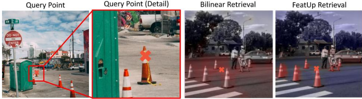
Figure 2.22: FeatUp can be used to improve the retrieval of small objects in cluttered scenes. A query image (left) is featured with DINO and a query point is selected. In the two images on the right, we compare the pixel similarity (the overlaid heatmap — red is similar, blue is dissimilar) and object retrieval (the \times ) produced by bilinear- vs. FeatUp-based algorithms. Because the scene is cluttered, bilinear interpolation blurs object features together and the resulting retrieval vector does not discriminate between ground and cones. FeatUp’s features better align with objects, allowing only the traffic cones to be retrieved.
