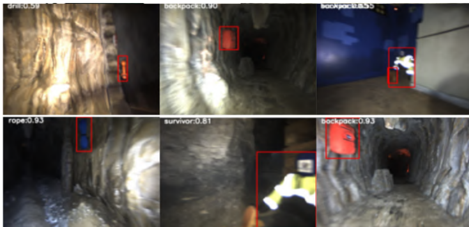
Figure 1.5: Examples of object detection and labels as produced by YOLOv3 Tiny [9], an approximately 63M-parameter [10] object detection model commonly used on mobile robotic platforms for its efficiency [7].
