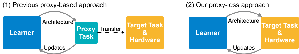
Figure 3.1: ProxylessNAS directly optimizes neural network architectures on target task and hardware. Benefiting from the directness and specialization, ProxylessNAS can achieve remarkably better results than previous proxy-based approaches. On ImageNet, with only 200 GPU hours ( 200 \times fewer than MnasNet [114]), our searched CNN model for mobile achieves the same level of top-1 accuracy as MobileNetV2 1.4 while being 1.8\times faster.
