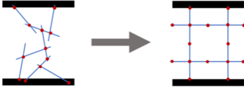
Figure 2.9: Two nanowire networks, one random (left) and one square grid (right). The cumulative length of nanowires in each network is equal, as are their areas, giving them equal density. In our formalism, then, they would have the same transparency and differences in the figure of merit arise purely from differences in electrical resistance.
