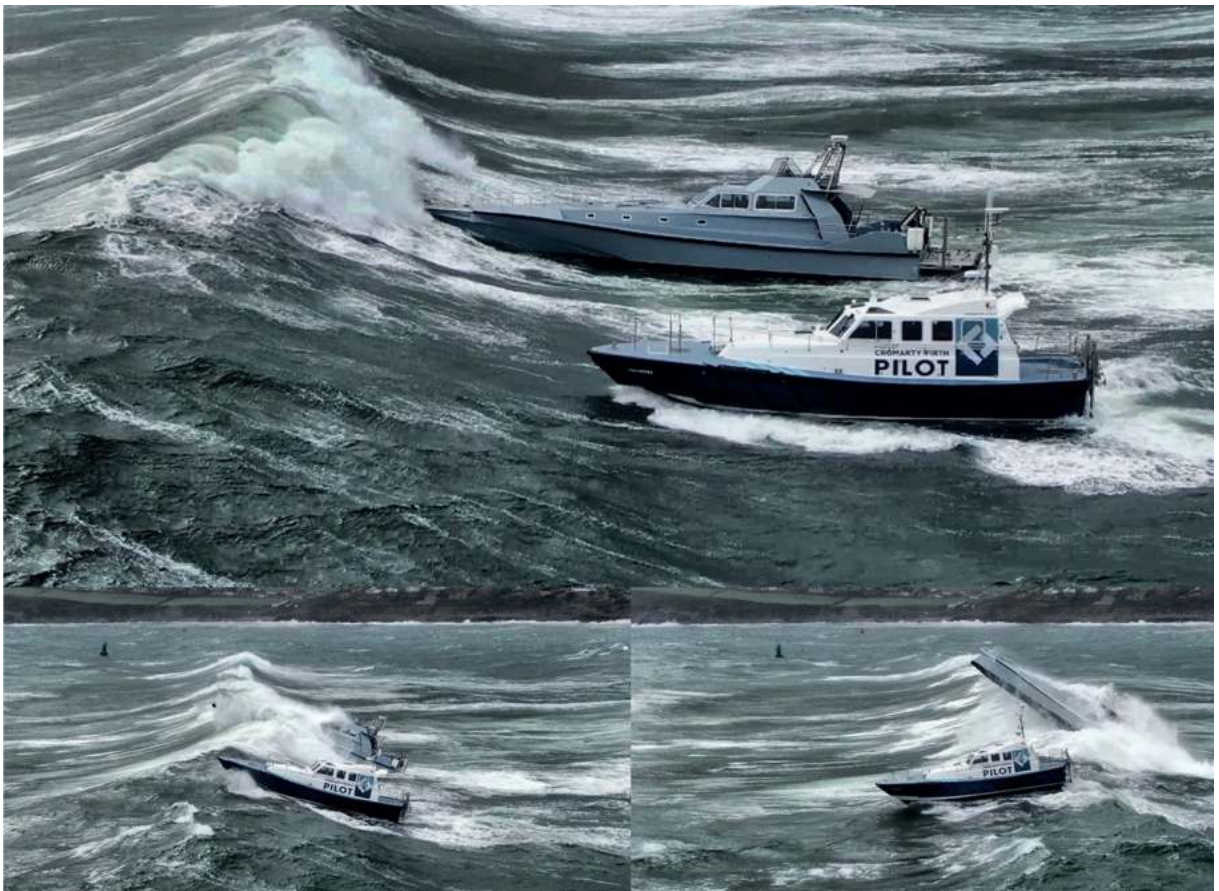
Figure 2-39: Differences when experiencing a breaking and a non-breaking waves are very large. Picture source is SAFEHAVEN MARINE and found in [268].
