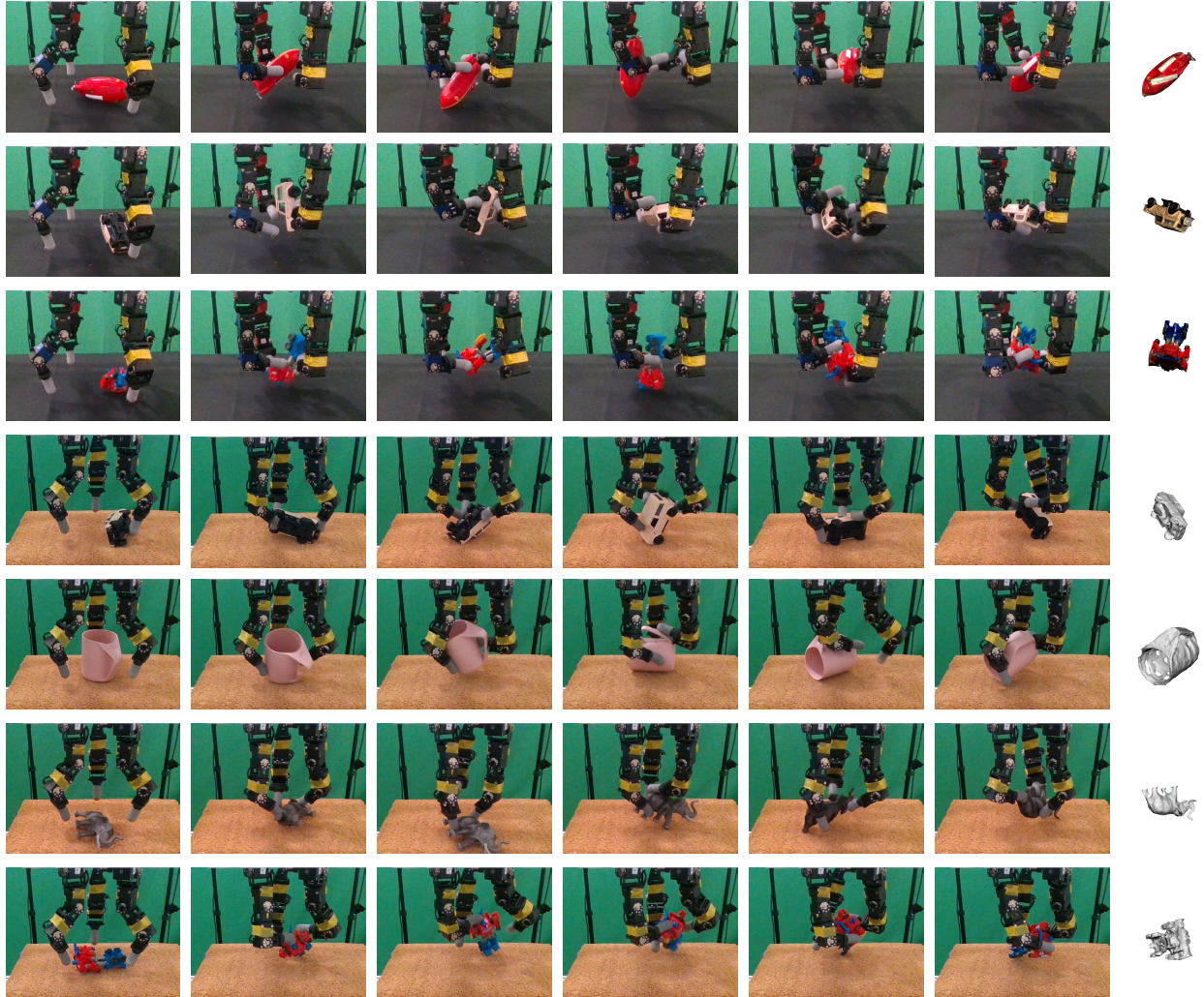
Figure 2.5: Reorientation of real objects. Examples of reorienting real objects that were not 3D printed using a four-fingered and a three-fingered manipulator.
