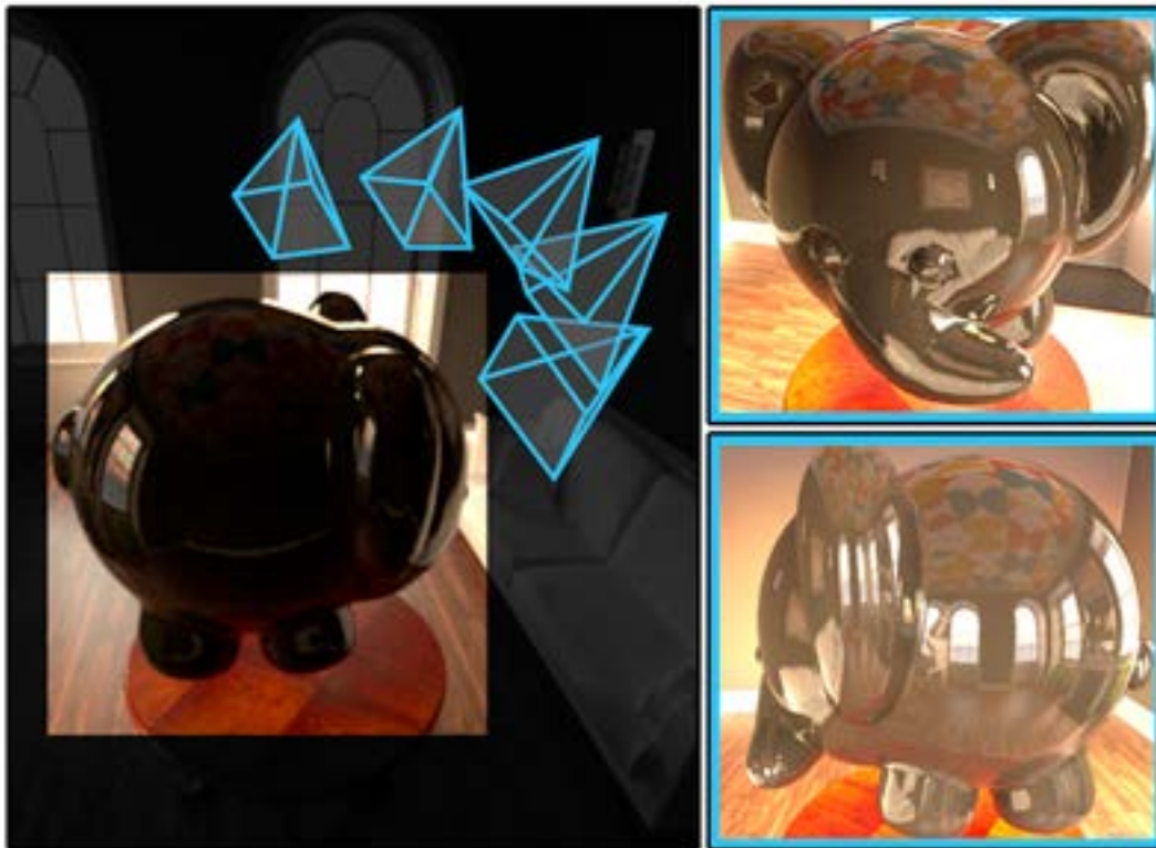
A new computer vision system turns any shiny object into a camera of sorts, enabling an observer to see around corners or beyond obstructions. Credit: Courtesy of the researchers
