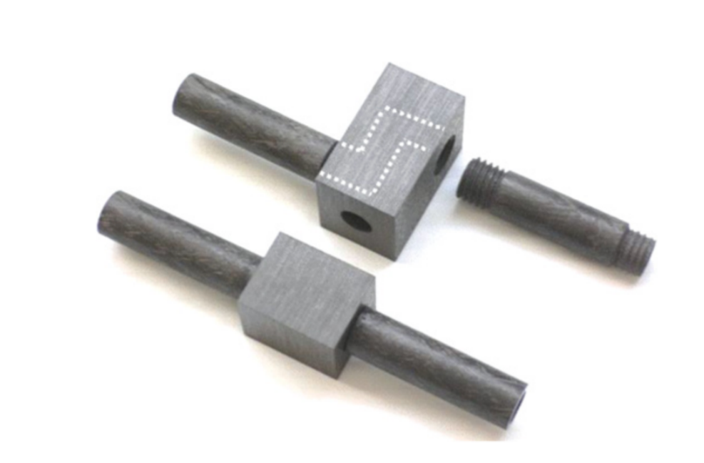
Figure 2.9: A threaded SiC/SiC joint. [31]
