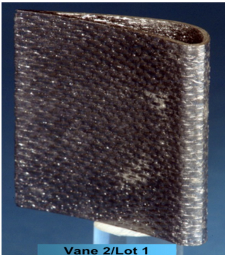
Figure 2.3: SiC/SiC turbine engine guide vane developed at NASA Glenn. [15]
