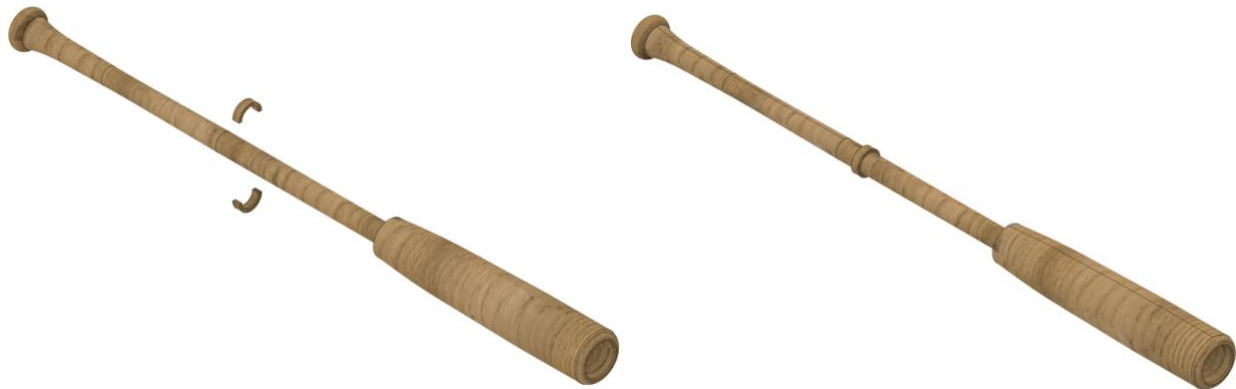
Figure 4.3: Ring stopper placement before and after attachment.
