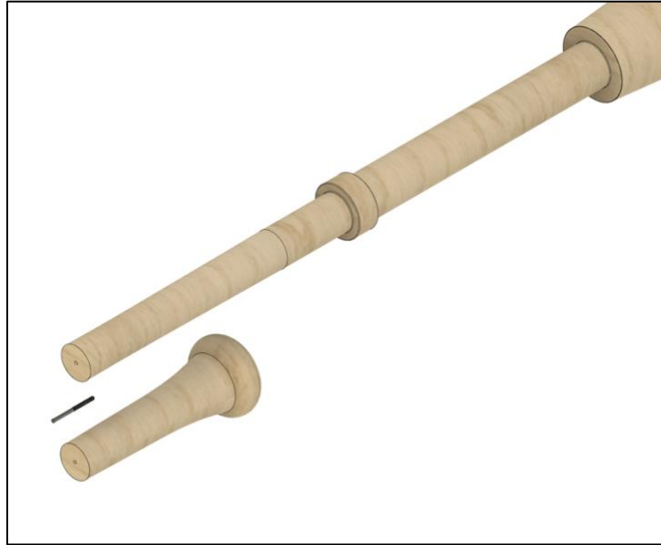
Figure 4.6: Three components of the handle detachability feature [18, 23].
