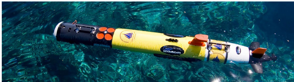
Figure 1: Figure 1 shows a top view of the REMUS 100 AUV designed at Woods Hole Oceanographic Institution (WHOI). The REMUS series contains a number of different versions rated for different depths [6].
