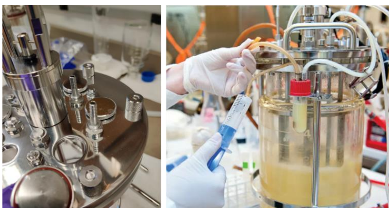
Figure 1.28: Left- standard ports on a bioreactor for probes including pH, oxygen and Raman, Right - a bioreactor with the probes introduced into the cell culture.
