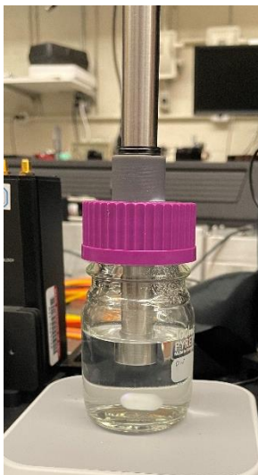
Figure 2.24: Immersion sleeve insertion setup for nitrate in water measurements with the sleeve inserted into a custom fabricated bottle cap to allow easy replacement of measured liquids without disturbing the probe.
