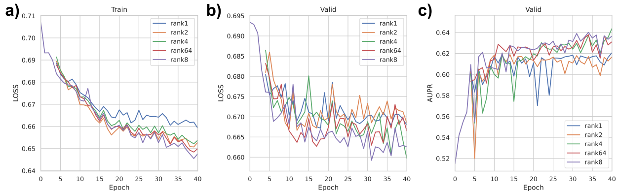
Figure D.3: Training (a) and validation (b) loss curves, AUPR (c) curves for models trained with LoRA ranks r = 1, 2, 4, 8, 64 from Table 6.5. Note that all other training parameters were held constant between these runs.
