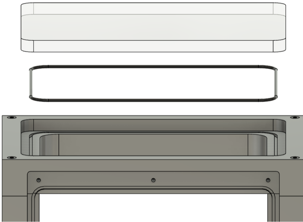
Figure 6-3: Exploded view of enclosure's top components and close-up of O-ring groove.
